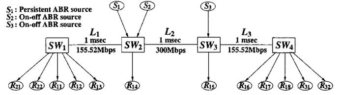
Fig. 5. Simulation model for multiple multicast VCs.
