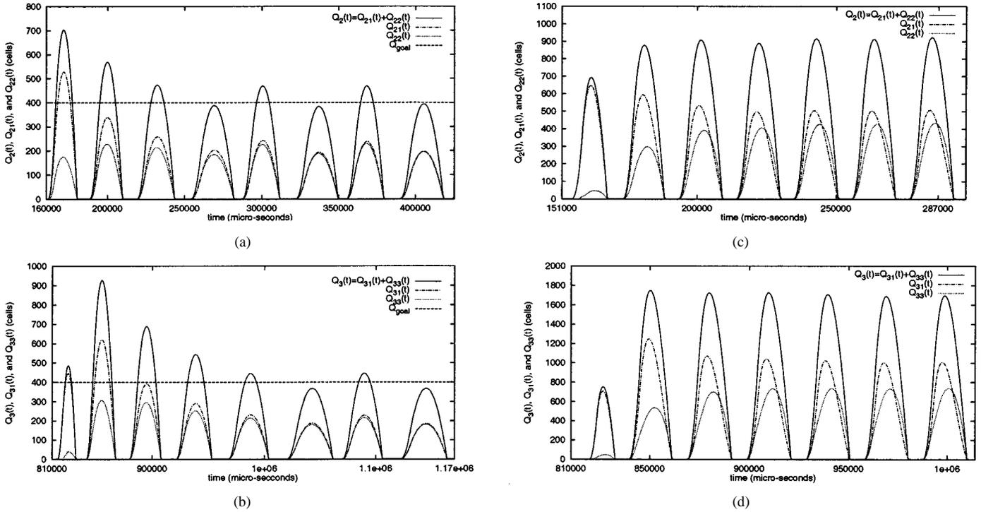
Fig. 7. Buffer occupancy fairness comparison between schemes with and without  $\alpha$ -control. (a) SW<sub>2</sub>:  $Q_{21}(t)$ ,  $Q_{22}(t)$  converge to fairness with  $\alpha$ -control. (b) SW<sub>3</sub>:  $Q_{31}(t)$ ,  $Q_{33}(t)$  converge to fairness with  $\alpha$ -control. (c) SW<sub>2</sub>:  $Q_{21}(t)$ ,  $Q_{22}(t)$  do not converge to fairness without  $\alpha$ -control. (d) SW<sub>3</sub>:  $Q_{31}(t)$ ,  $Q_{33}(t)$  do not converge to fairness without  $\alpha$ -control.
