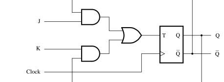
7.9. This circuit acts as a negative-edge-triggered JK flip-flop, in which J = A, K = B, Clock = C, Q = D, and  $\overline{Q} = E$ . This circuit is found in the standard chip called 74LS107A (plus a *Clear* input, which is not shown).
