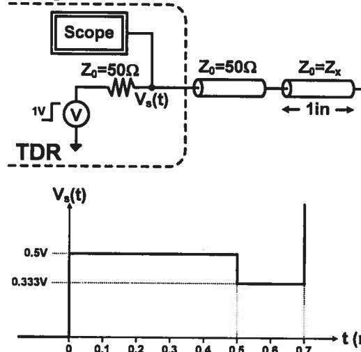
$Z_x$  impedance discontinuity is detected at TDR at  $t = 0.5\text{ns}$
