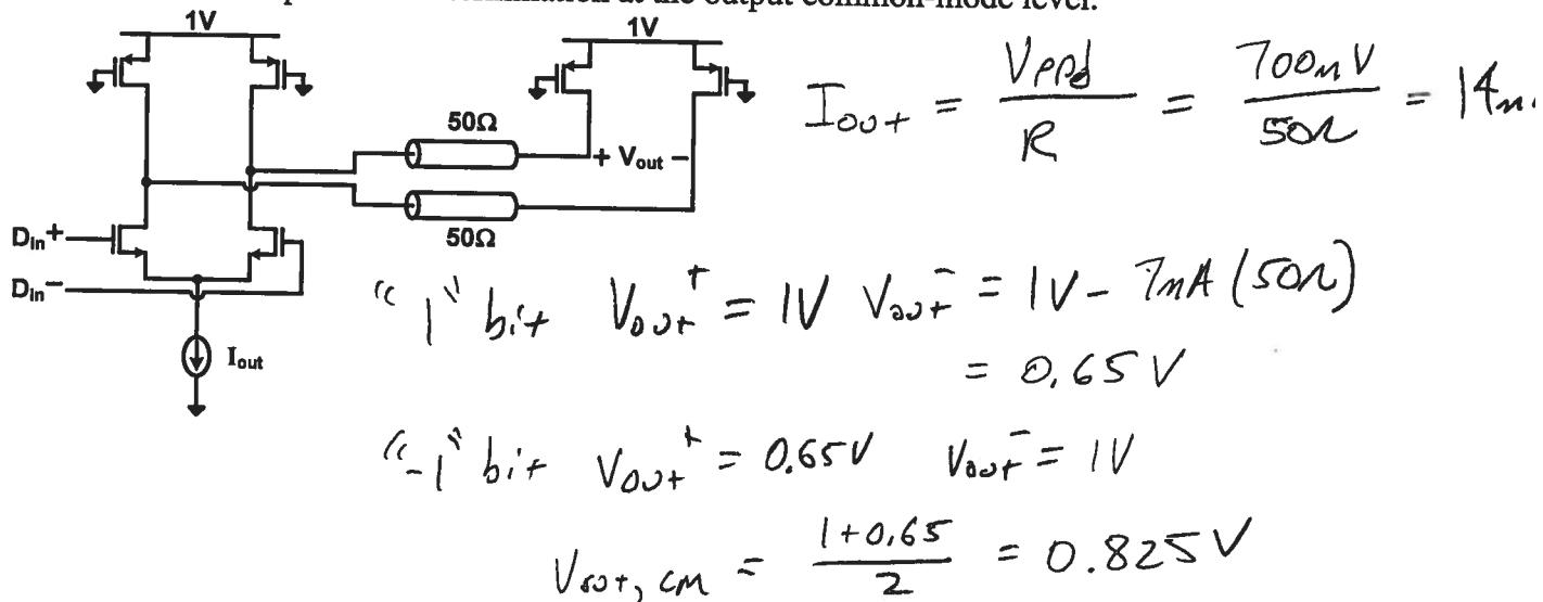
\* Sizing PMOS termination at common-mode level
