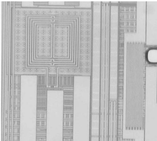
**Fig. 16** Micro-photograph displaying the  $85\ \mu\text{m} \times 85\ \mu\text{m}$  differential, interleaved spiral inductors (left) and a single metal-insulator-metal capacitor (right)
