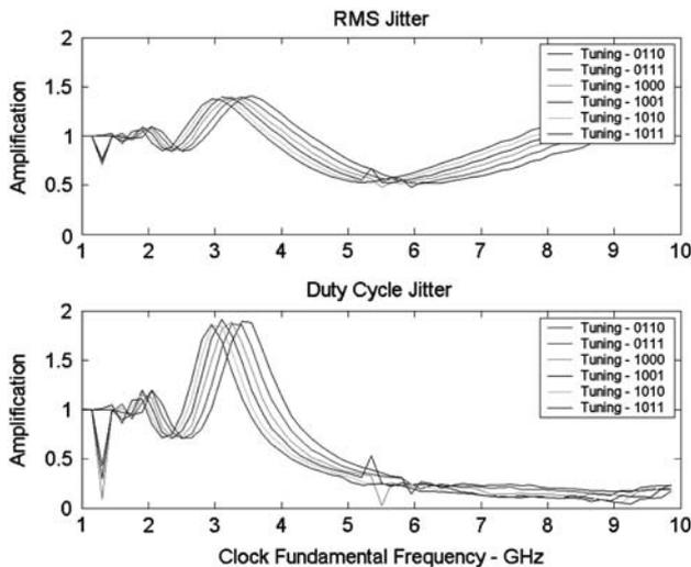
**Fig. 19** Simulated jitter amplification versus filter center frequency tuning
