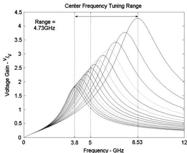
Fig. 18 4-bit tuning range of the proposed bandpass filter
