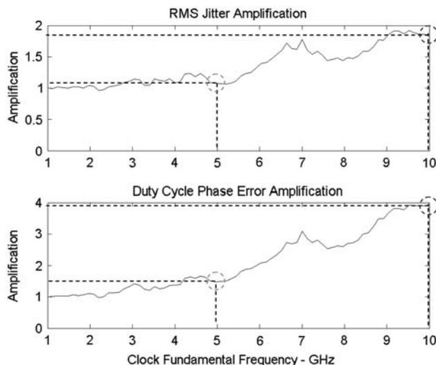
**Fig. 6** Anticipated random jitter and DCD amplification at various clock frequencies for a six inch channel across an FR4-based printed circuit board
