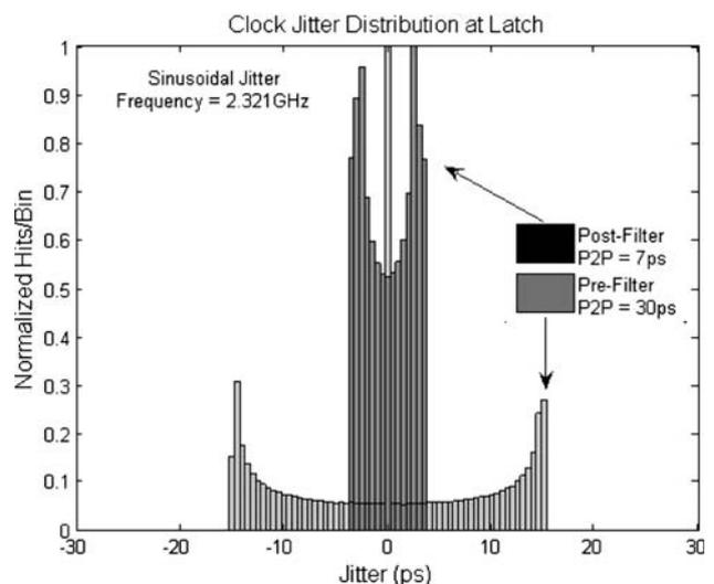
**Fig. 22** Simulated impact of the proposed bandpass filter circuit on a sinusoidal jitter component
