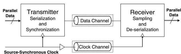
**Fig. 1** A simplified source-synchronous link illustrating the relationship between the forwarded-clock and the data throughout the interconnect system
