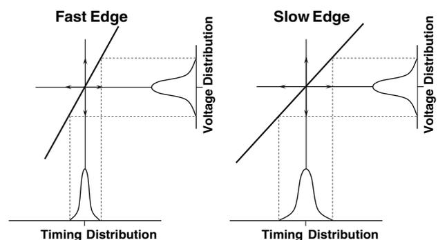
**Fig. 4** Illustration of the translation of random noise to random jitter through the slew-rate of the associated signal
