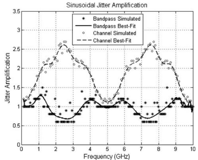
**Fig. 13** Sinusoidal jitter amplification of the proposed bandpass filter with clock frequency fixed at 5 GHz and sinusoidal jitter frequency swept from 100 MHz to 10 GHz
