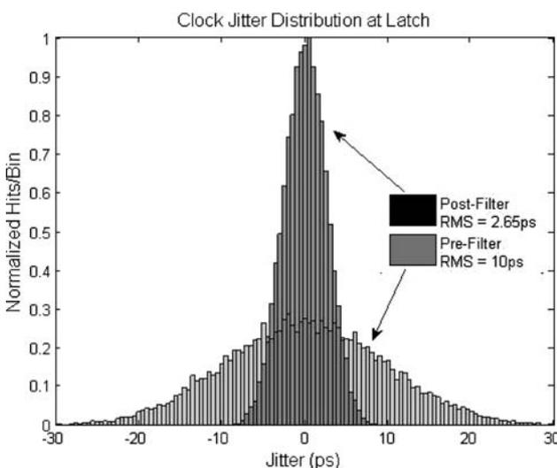
**Fig. 20** Simulated impact of the proposed bandpass filter circuit on random jitter
