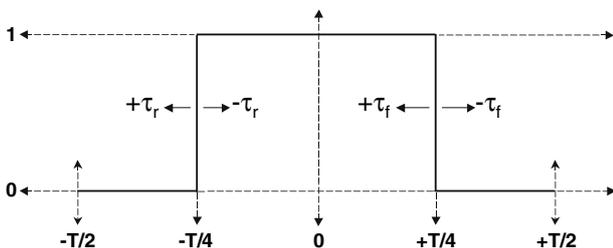
Fig. 11 Waveform used in the derivation of the Fourier series representing a clock with DCD
