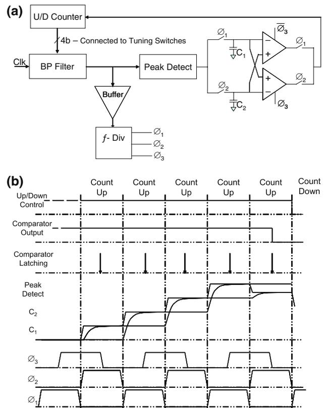
**Fig. 17** Peak Tuning: (a) Block diagram of a center frequency tuning scheme based on peak detection; (b) Waveforms corresponding to the calibration algorithm
