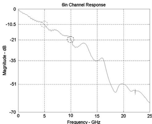
**Fig. 5** Target clock channel frequency response for a six inch channel across an FR4-based printed circuit board
