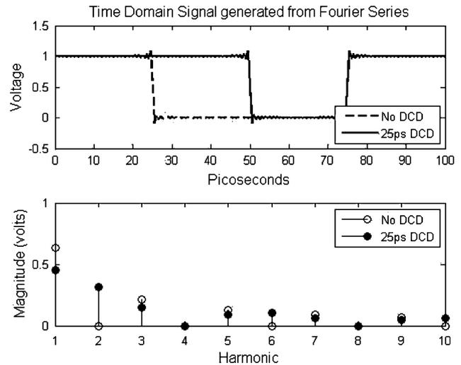
Fig. 12 The upper window presents an ideal clock waveform compared with a clock exhibiting 25 ps of DCD by delaying the falling edge of the second waveform through the parameterized Fourier series just derived. The lower window presents the resulting variation in the 10 GHz fundamental and the first nine higher order harmonics, illustrating the high frequency nature of jitter due to duty cycle error
