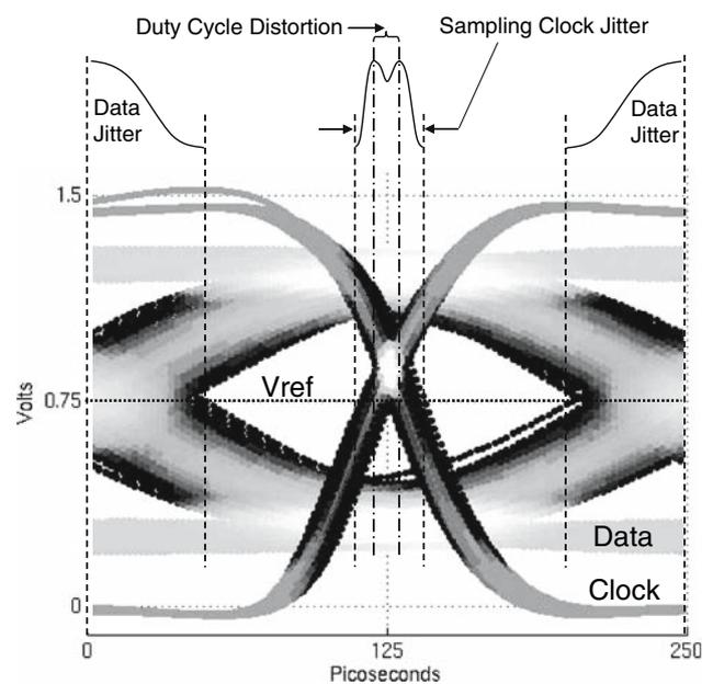
**Fig. 8** Eye diagram illustrating the effects of both clock and data jitter on timing margin. Duty cycle distortion produces the bimodal sampling clock distribution
