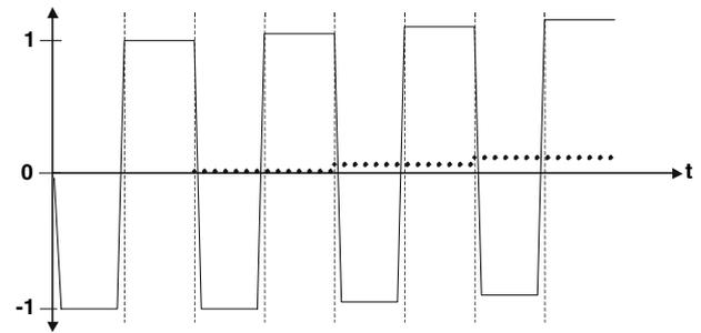
**Fig. 10** Illustration of how DCD in a signal accumulates across a lowpass channel
