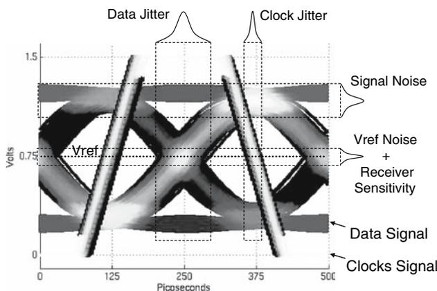
**Fig. 3** Illustration of the combined impact of data and clock jitter on timing margin
