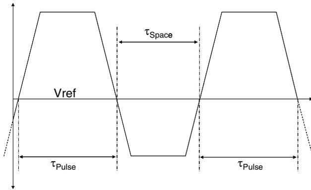
**Fig. 9** Illustration of how the addition of any amount of DC offset voltage to a perfectly symmetric, finite rise/fall time, square wave generates duty cycle error
