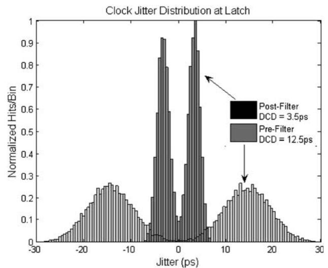
**Fig. 21** Simulated impact of the proposed bandpass filter circuit on DCD
