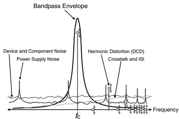
**Fig. 2** High-level frequency domain illustration of the impact that a bandpass filter should have on the spectral components of clock degrading noise
