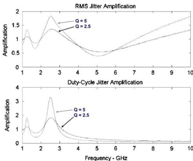
**Fig. 7** Anticipated random jitter and DCD amplification for two bandpass filters with Qs of 2.5 and 5
