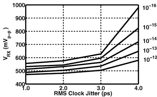
Fig. 29. BER curves for different combination of received swings and clock jitter.
