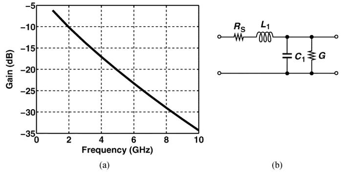
Fig. 24. (a) Loss profile of 30-in microstrip on FR4 board. (b) Narrowband loss model.
