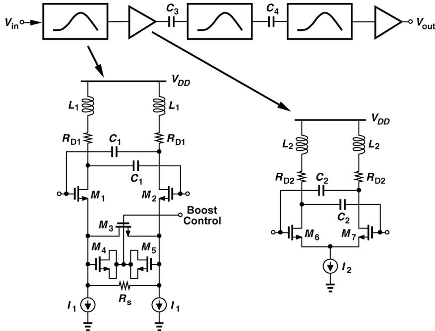
Fig. 6. Equalizer filter I with reverse scaling.
