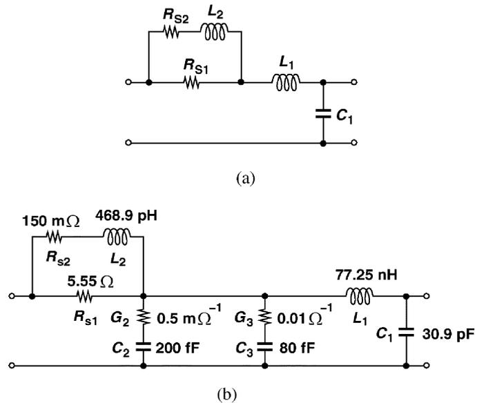
Fig. 25. (a) Model for variable skin effect. (b) Proposed broadband model for a 1-in trace.
