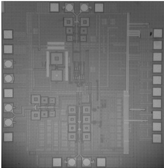
Fig. 20. Die photograph of merged adaptive equalizer/CDR.
