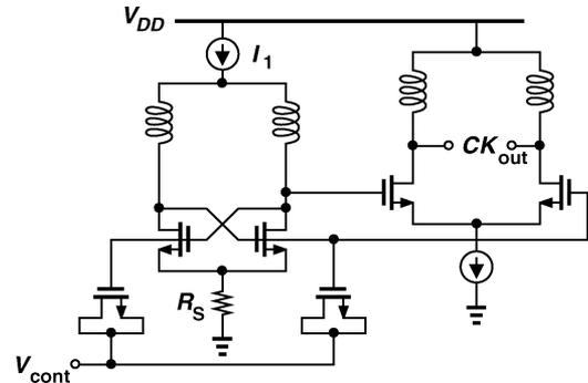
Fig. 16. VCO and buffer circuit.
