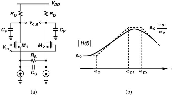
Fig. 2. RC-degenerated differential pair. (a) Circuit implementation. (b) Frequency response: actual response (solid line); bode approximation (dashed line).
