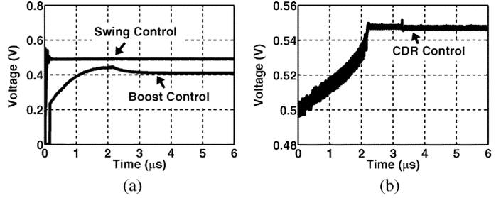
Fig. 14. Simulated dynamics of (a) boost and swing control signals, and (b) the control voltage of the VCO in the CDR loop.
