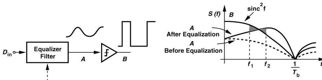
Fig. 10. Spectrum before and after slicer with swing mismatch.
