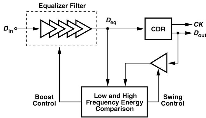
Fig. 13. Proposed merged adaptive equalizer/CDR architecture.
