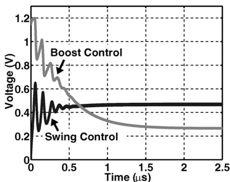
Fig. 11. Simulated dynamics of the swing and boost control loops.
