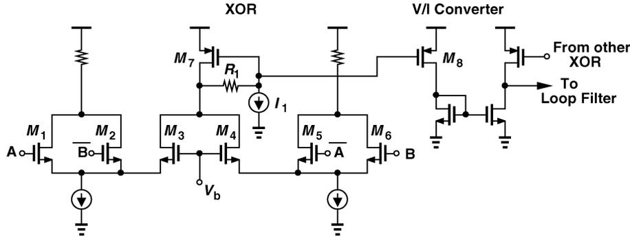
Fig. 17. XOR and  $V/I$  circuit.
