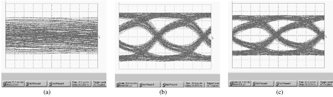
Fig. 21. Measured results before and after equalization/data recovery at 10 Gb/s for FR4 traces (horizontal scale: 20 ps/div.): (a) before equalization/data recovery for 24-in FR4 (horizontal scale: 10 ps/div., vertical scale : 75 mV/div.), (b) after equalization/data recovery for 24-in FR4 (horizontal scale: 20 ps/div., vertical scale : 20 mV/div.), (c) after equalization/data recovery for 6-in FR4 (horizontal scale: 20 ps/div., vertical scale: 20 mV/div.).
