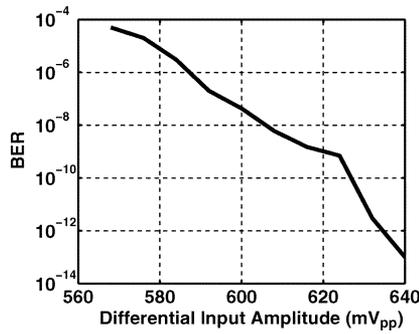
Fig. 22. BER sensitivity graph for equalization/data recovery for 24-in FR4 at 10 Gb/s.
