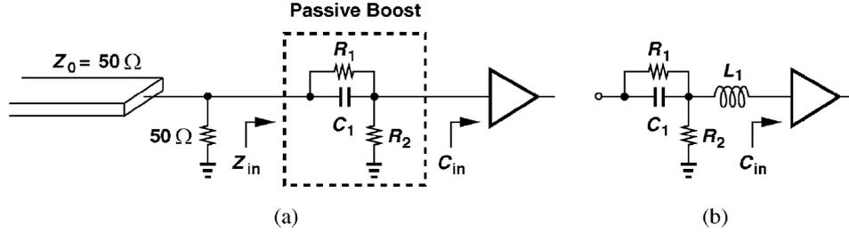
Fig. 3. (a) Passive network. (b) Proposed passive network with series inductive peaking.
