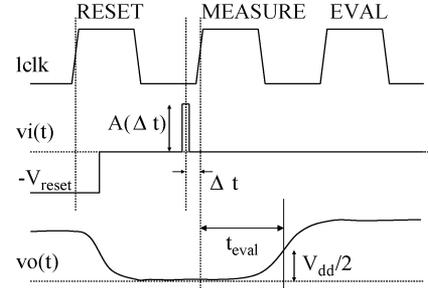
Fig. 27. Signal diagram for latch transfer function extraction procedure.
