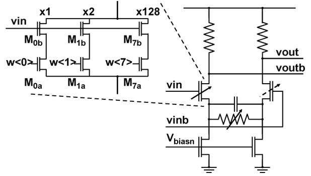
Fig. 4. Schematic of the proposed voltage shifting amplifier.
