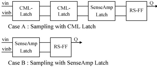
Fig. 12. Data paths for latch comparison.
