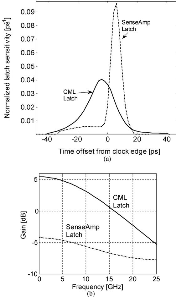
Fig. 13. (a) Latch sensitivity function for CML latch (solid) and SenseAmp latch (dotted). (b) Latch transfer function for CML latch (solid) and SenseAmp latch (dotted) at a target sensitivity of 5 mV.
