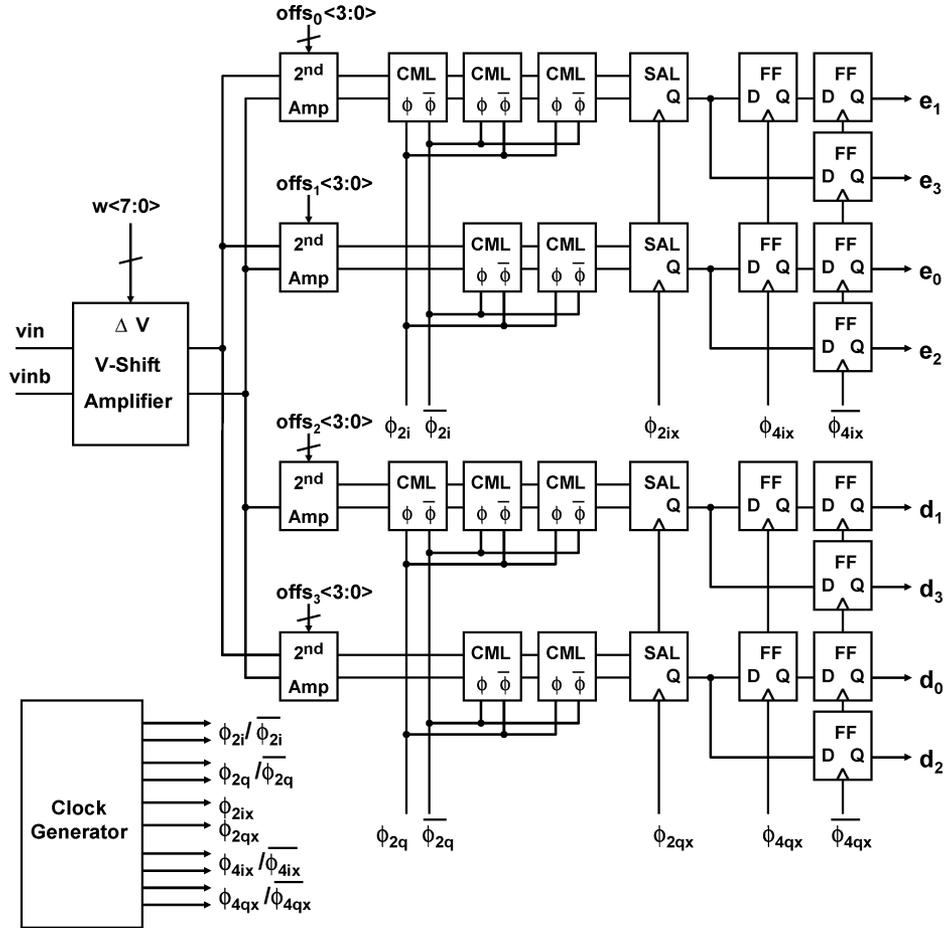
Fig. 14. Architecture of the 1:4 demux slice.
