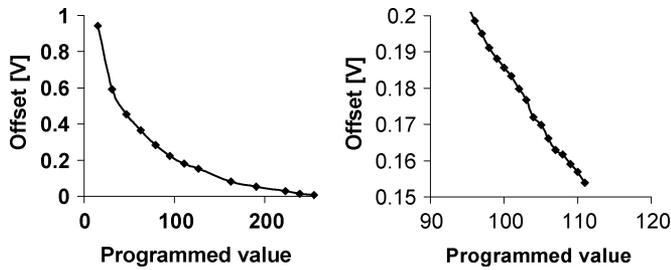
Fig. 20. Measured offset voltage versus programmed value of the V-shifting amplifier. Global characteristic (left) and detail (right).
