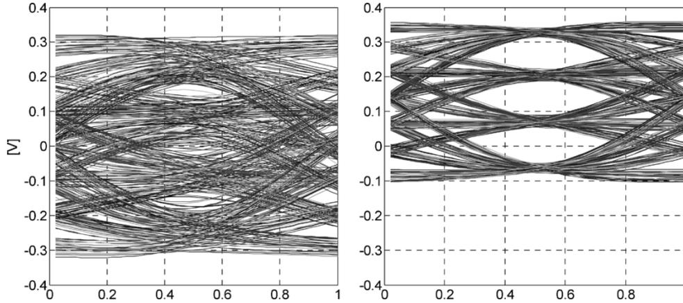
Fig. 6. Combined effect of voltage shift and equalization. Eye diagram at the input (left) and output (right) of the amplifier.
