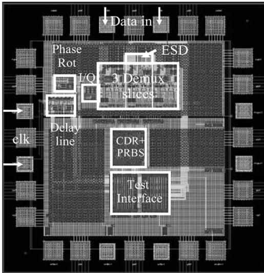
Fig. 26. Layout of the PAM-4 receiver.
