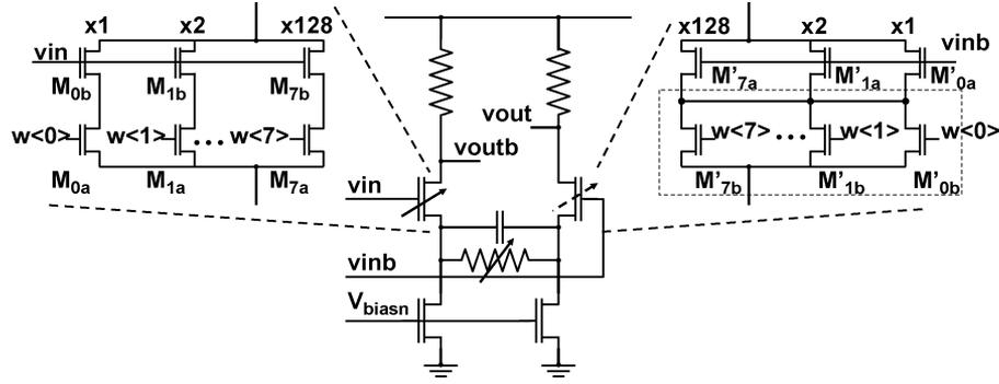
Fig. 8. Voltage shifting amplifier with improved common-mode rejection.
