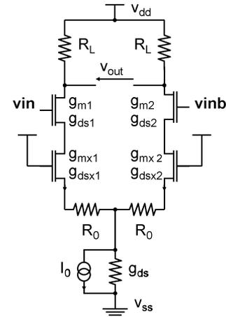
Fig. 7. Schematic used to derive small-signal gains.
