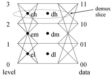
Fig. 2. PAM-4 eye diagram and the required sampling points.
