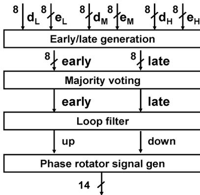
Fig. 19. Data flow in the digital CDR logic.
