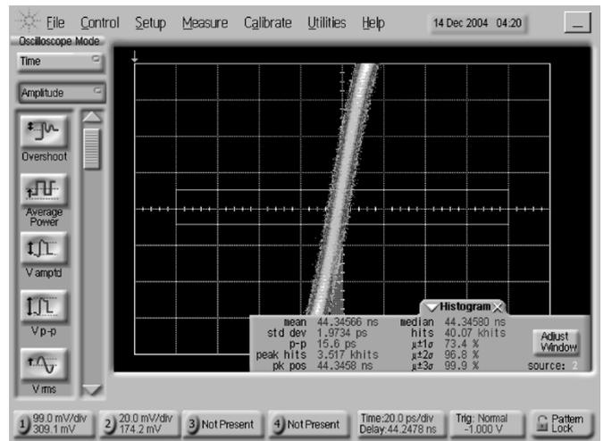
Fig. 24. Recovered clock from input data with 350 ppm frequency offset between data and receiver clock.
