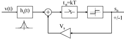
Fig. 10. Proposed sampling latch model.
