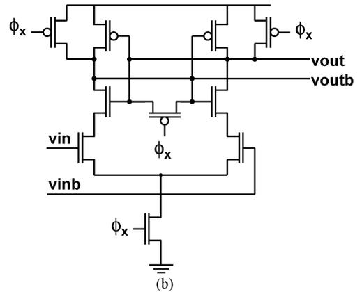
Fig. 11. Comparison of (a) CML-sampling latch and (b) SenseAmp-style latch for analog sampling.
