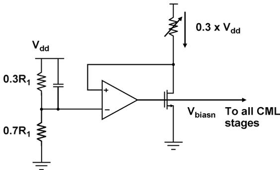
Fig. 16. Biasing concept with variable resistor.
