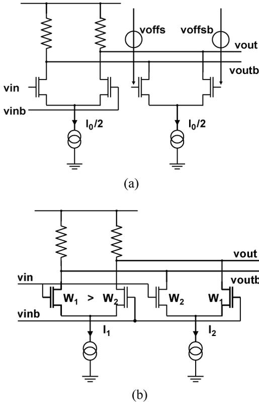
Fig. 3. Existing solutions for voltage shifting amplifiers.
