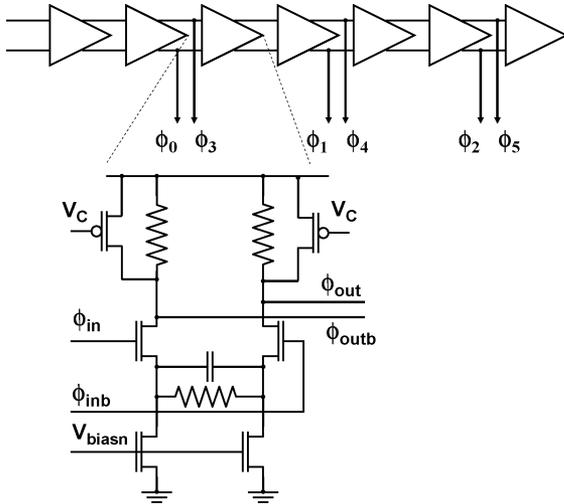
Fig. 17. Delay line with capacitive source degeneration.
