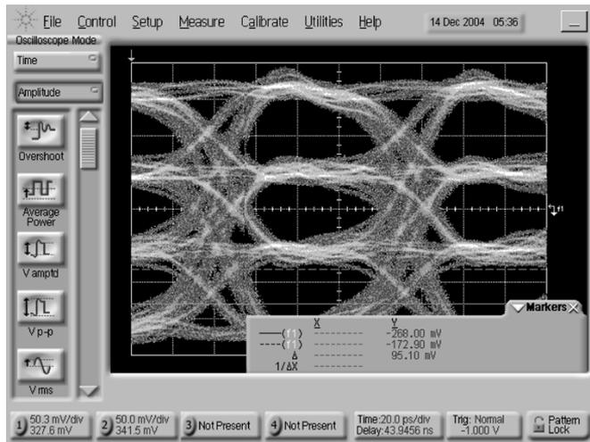
Fig. 22. PAM-4 eye diagram of the input data.
