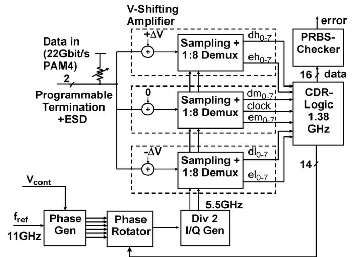
Fig. 1. Architecture of the PAM-4 receiver.
