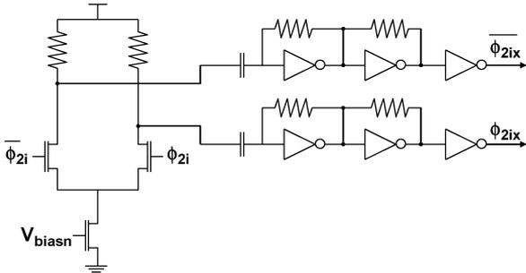
Fig. 15. Differential to single-ended converter.
