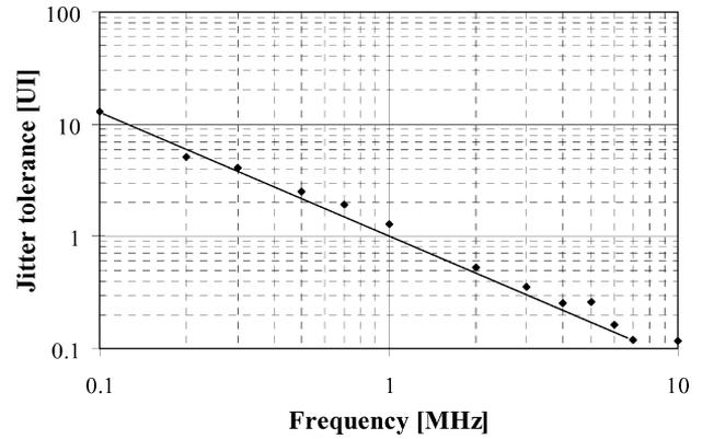
Fig. 23. Jitter tolerance at BER =  $10^{-12}$ .
