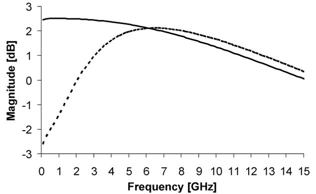
Fig. 5. Transfer function of the voltage shifting amplifier without (solid) and with (dashed) capacitive source degeneration.
