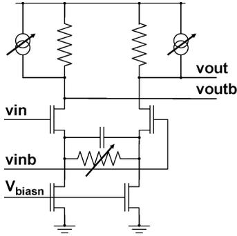
Fig. 9. Schematic of the second amplification stage providing per-latch offset compensation.
