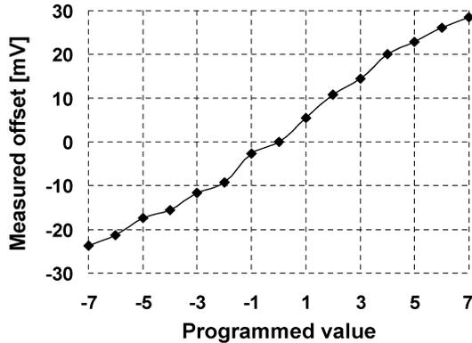
Fig. 21. Measured latch offset compensation capability.
