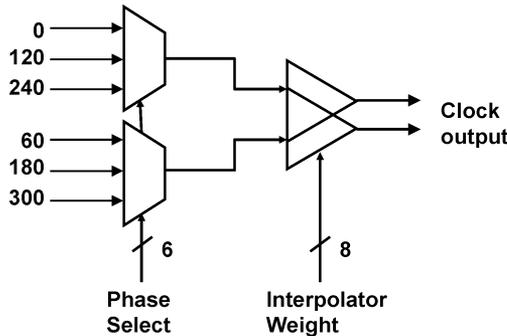
Fig. 18. Phase rotator implementation.
