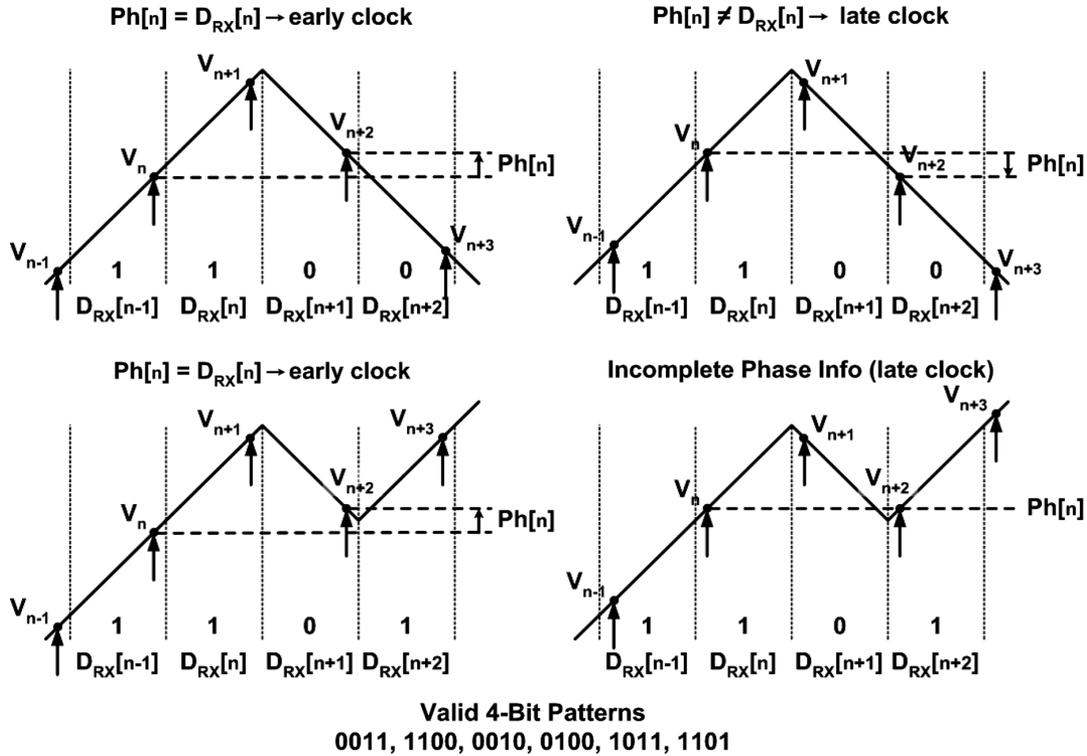
Fig. 10. Input voltage waveform with baud-rate phase detection [35].
