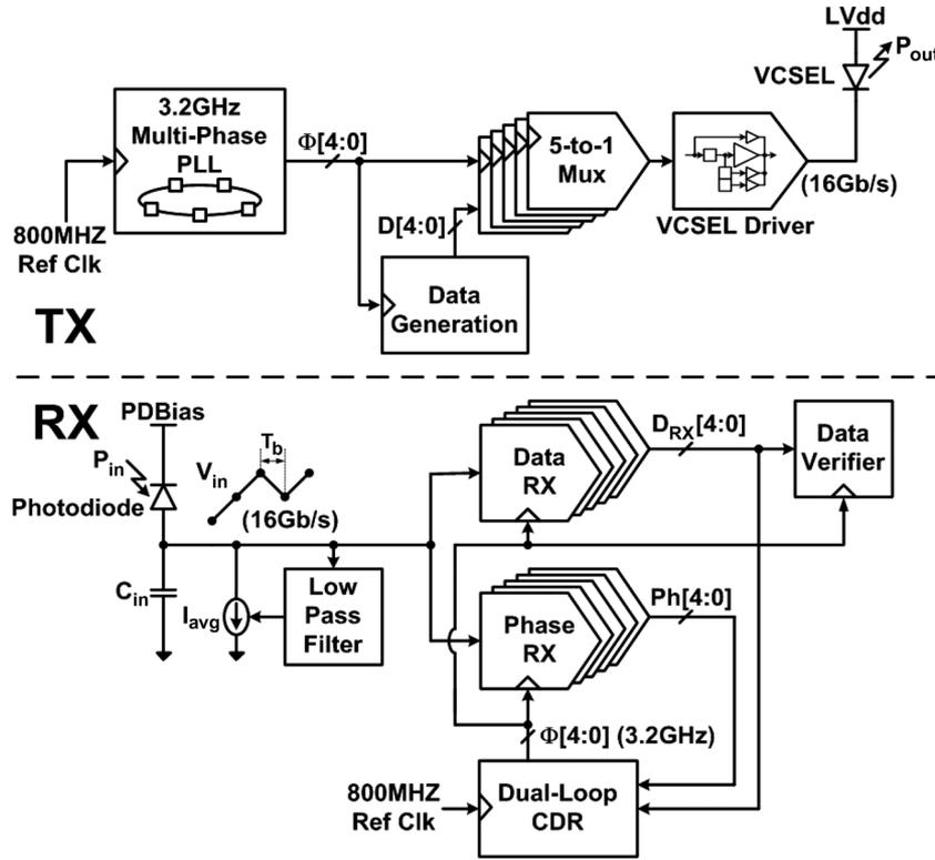
Fig. 2. Optical transceiver architecture.
