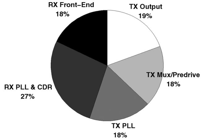
Fig. 18. Optical transceiver power breakdown at 16 Gb/s.
