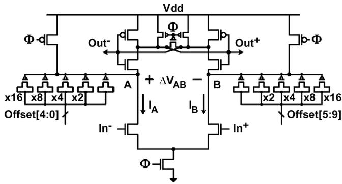
Fig. 8. Sense amplifier with capacitive offset correction.
