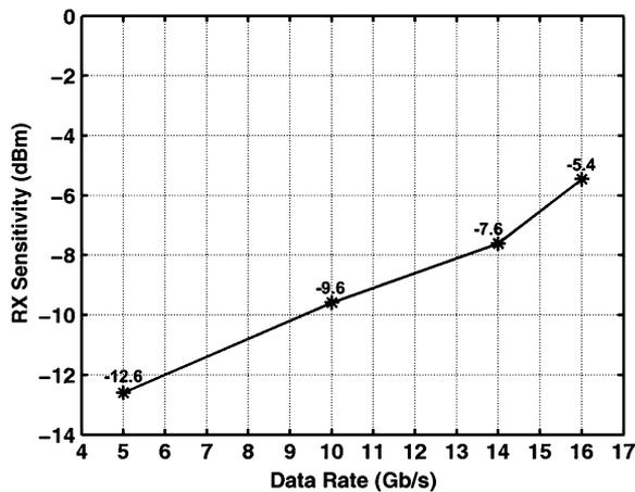
Fig. 16. Measured integrating receiver sensitivity versus data rate.
