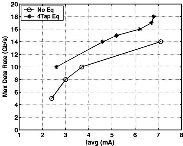
Fig. 6. VCSEL transmitter maximum data rate versus average current.
