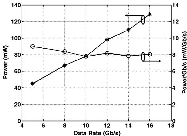
Fig. 17. Optical transceiver power versus data rate.
