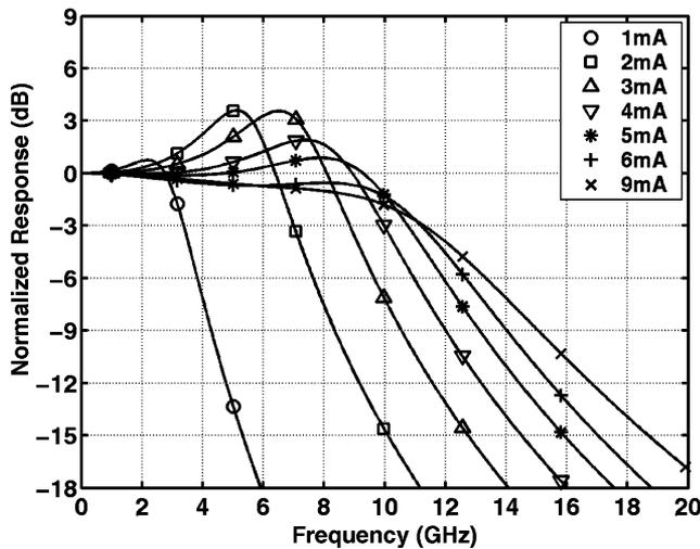
Fig. 3. Modeled 10 Gb/s class VCSEL frequency response [22].
