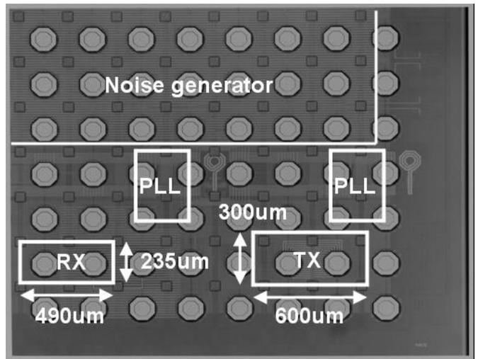
Figure 3.6.6: Chip micrograph.
