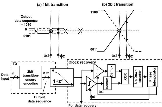
Figure 3.6.5: Clock recovery in duobinary signaling.
