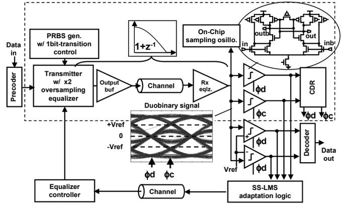
Figure 3.6.2: Block diagram of duobinary signaling system.
