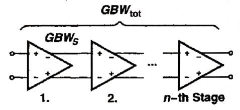
a) Design the limiting amplifier to achieve a 26dB total gain and 25GHz total bandwidth with the minimum per-stage gain-bandwidth product. Give the stage number and the per-stage gain and bandwidth. Also compute the per-stage gain-bandwidth product.
