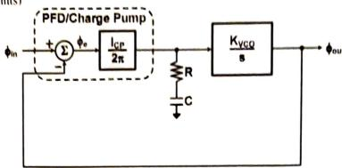
a) For the PLL block diagram shown above, find the expressions for the forward path gain G(s) and the closed-loop transfer function  $H(s)=\phi_{out}(s)/\phi_{in}(s)$ . (10 points)
