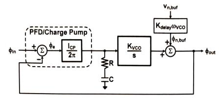
a) Find the expression for the post-VCO buffer voltage noise induced phase noise transfer function,  $T(s) = \phi_{out}(s)/v_{n,buf}(s)$ . (15 points)
