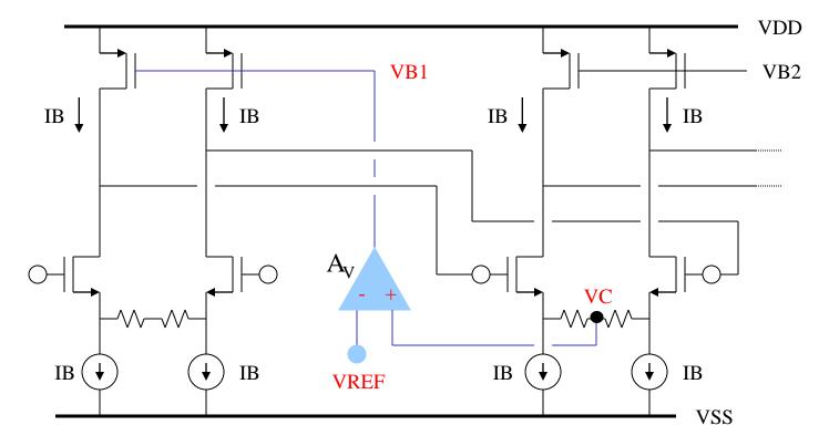
Common-mode loop gain =  $A_V Gm_p R_L$ 3 poles in the CMFB loop. Loop stability requires  $A_V Gm_p / C_L < \omega_{p2} @ VC, \omega_{p3} @ VB1$
