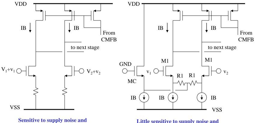
Sensitive to supply noise and common-mode input signals
