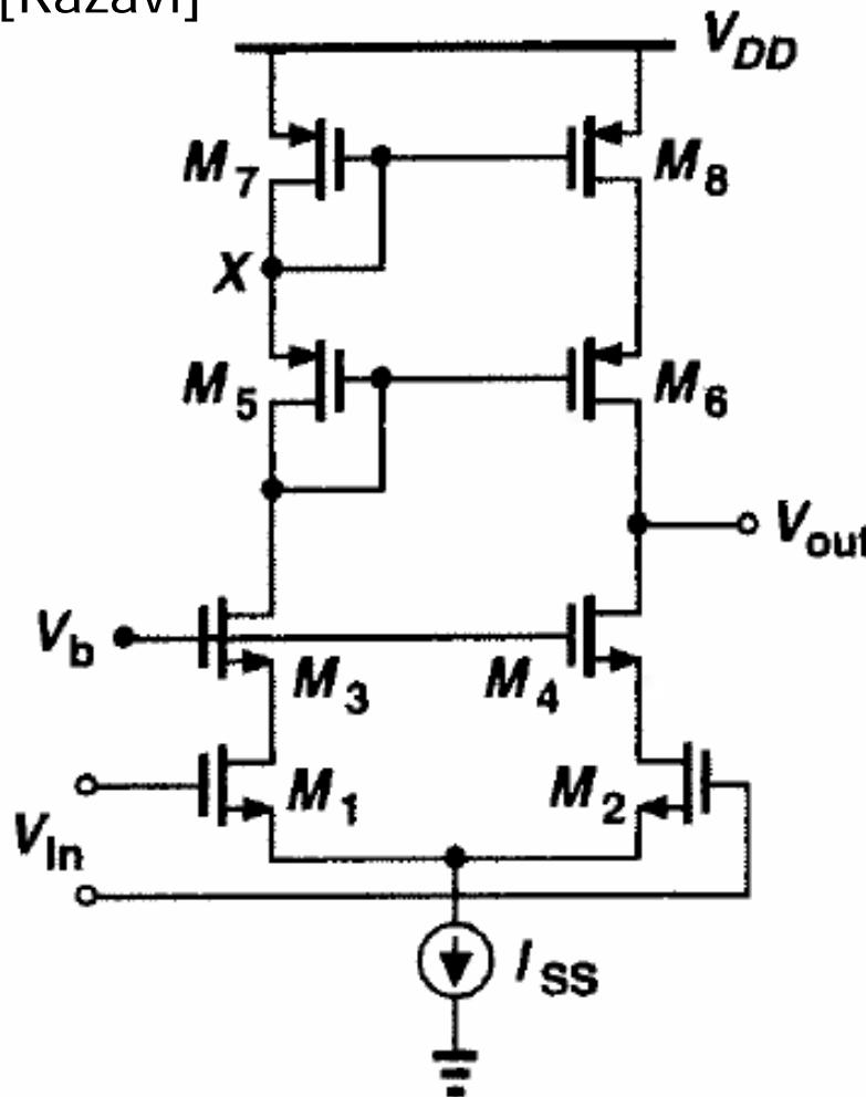
$$\text{DC Gain } A_v = G_m R_{out} \approx g_{m1} (g_{m4} r_{o2} r_{o4} \parallel g_{m6} r_{o8} r_{o6})$$
