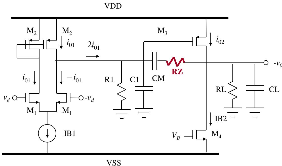
$$A(s) = \frac{A_{VDC} \left(1 - \frac{s}{\omega_z}\right)}{\left(1 + \frac{s}{\omega_{p1}}\right) \left(1 + \frac{s}{\omega_{p2}}\right) \left(1 + \frac{s}{\omega_{p3}}\right)}$$
