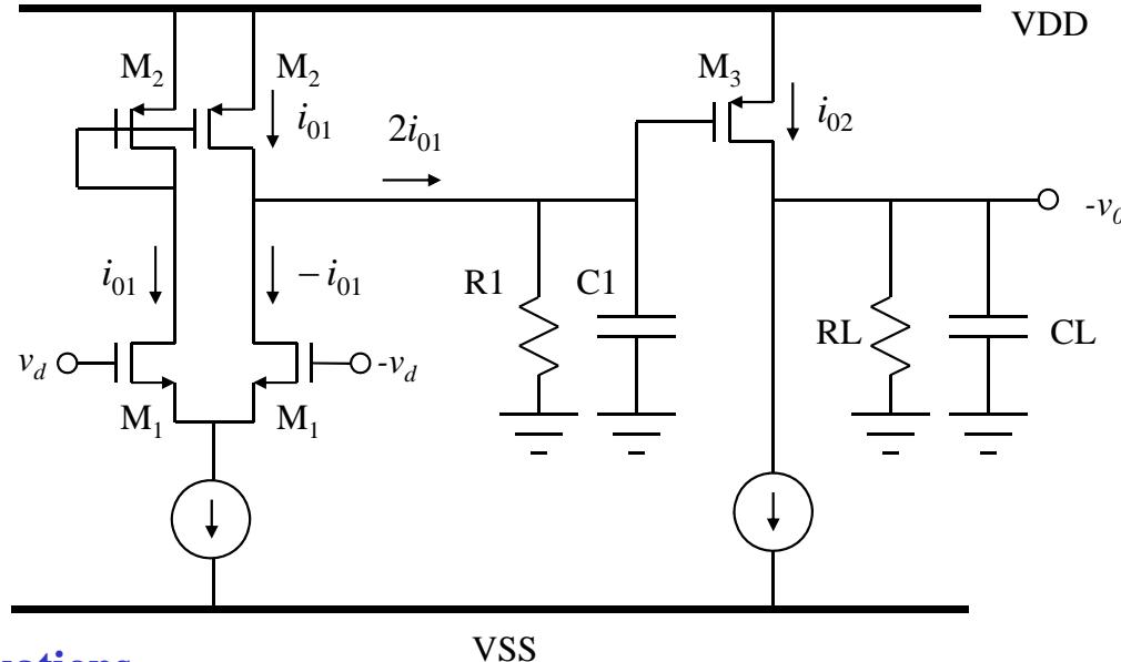
$$A(s) = \frac{A_{VDC}}{\left(1 + \frac{s}{\omega_{p1}}\right)\left(1 + \frac{s}{\omega_{p2}}\right)}$$
