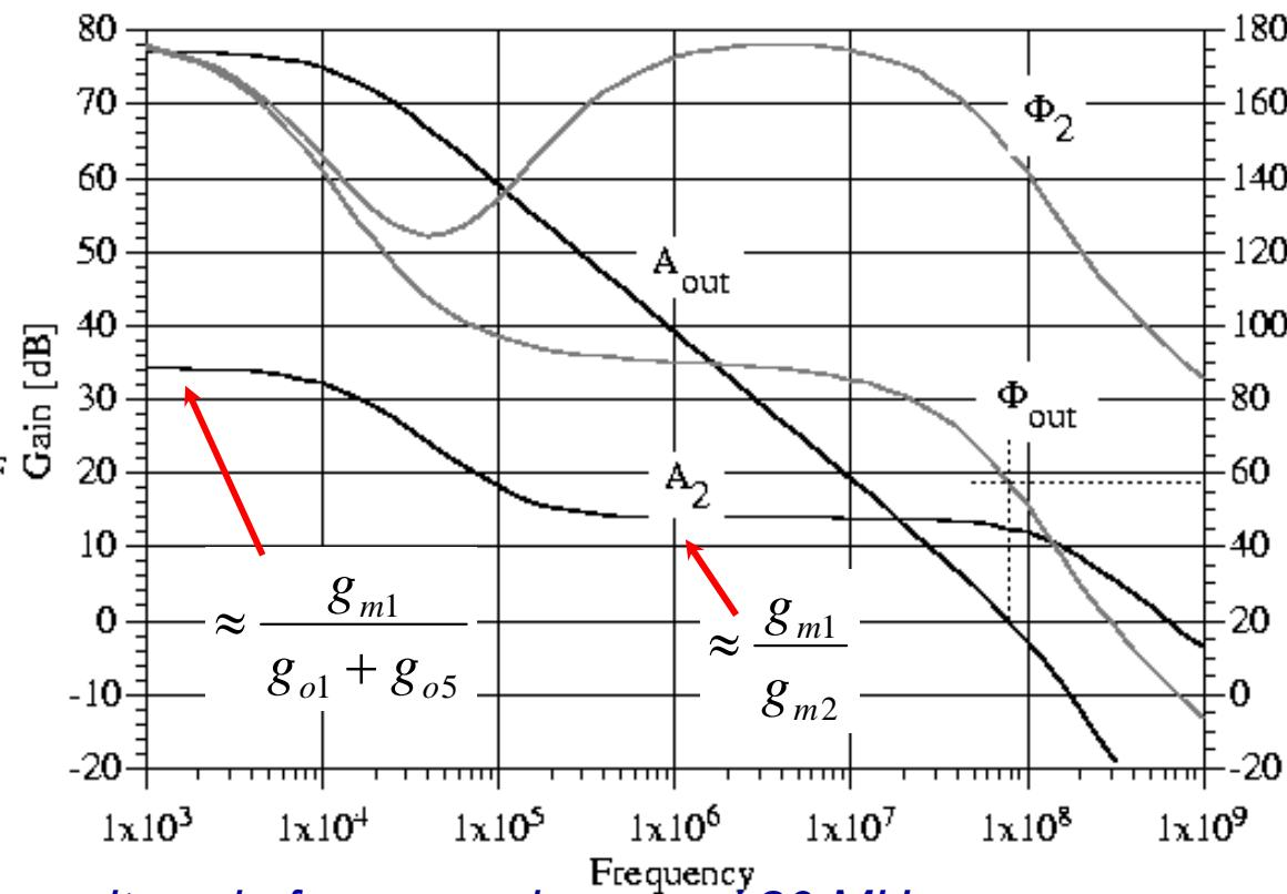
The low frequency gain is 77 dB and the unity gain frequency is around 80 MHz.
