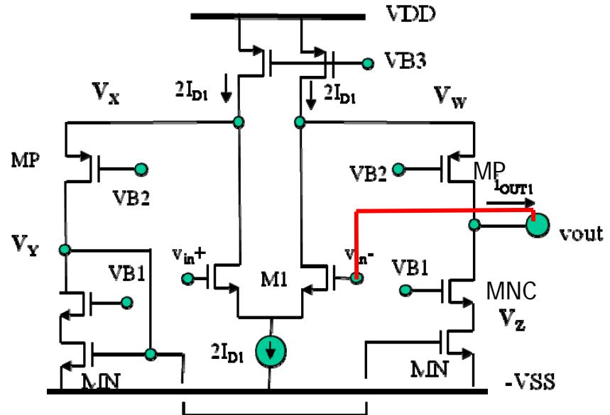
**Maximum  $V_{out}$  set by MP saturation**
