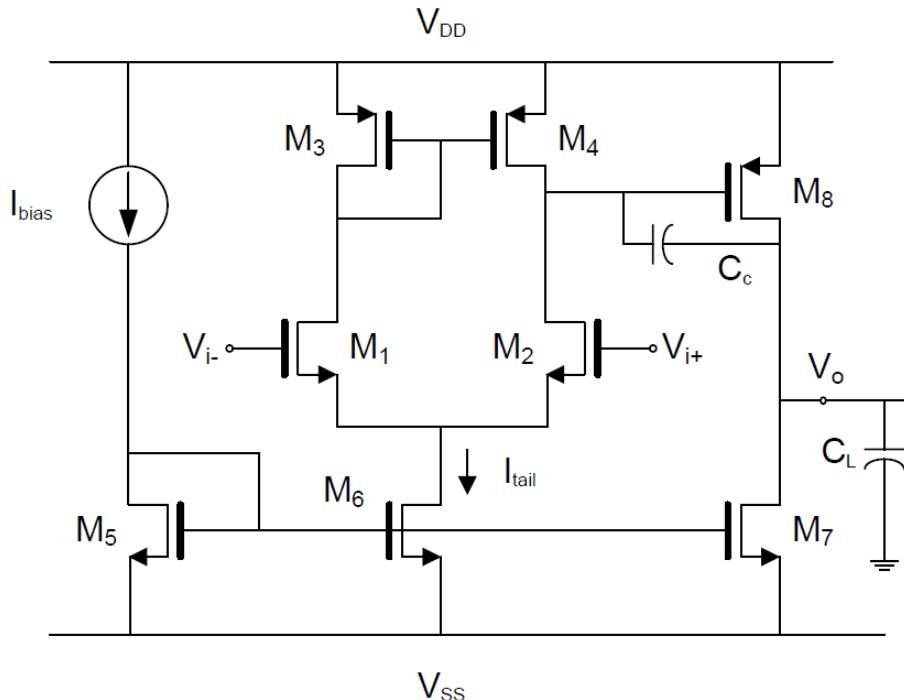
**DC Gain**  $A_{VDC} = A_{v1}A_{v2} = \left( -\frac{g_{m2}}{g_{o2} + g_{o4}} \right) \left( -\frac{g_{m8}}{g_{o8} + g_{o7}} \right) = \frac{g_{m2}g_{m8}}{(g_{o2} + g_{o4})(g_{o8} + g_{o7})}$
