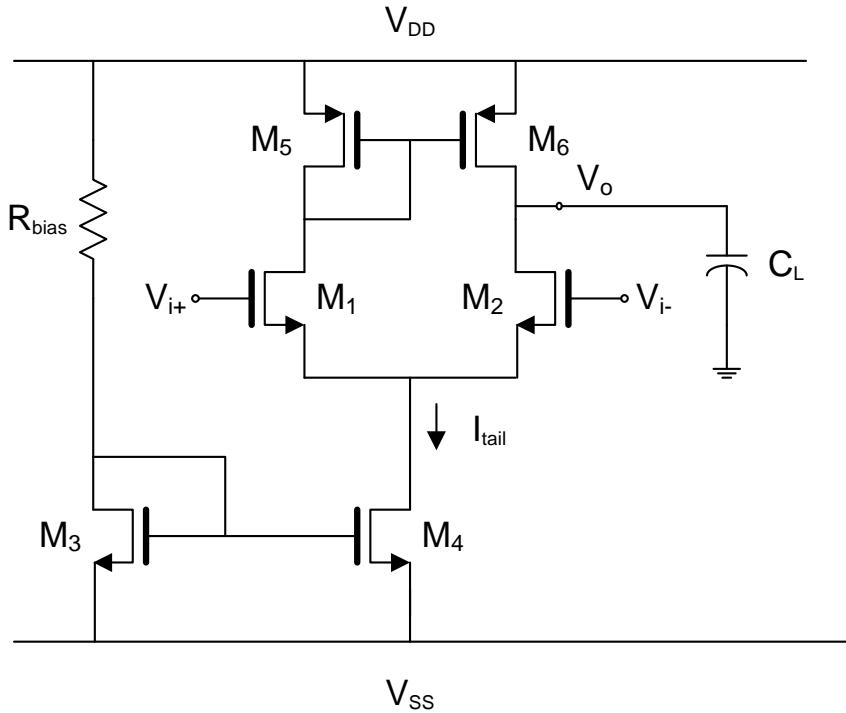
$$\text{DC Gain } A_v = G_m R_{out} = g_{m1} (r_{o2} \parallel r_{o6})$$
