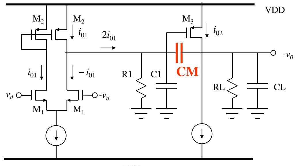
$$\text{Phase\_margin} = 180 - \tan^{-1}\left(\frac{\omega_u}{\omega_{p1}}\right) - \tan^{-1}\left(\frac{\omega_u}{\omega_{p2}}\right) - \boxed{\tan^{-1}\left(\frac{\omega_u}{\omega_{ZERO}}\right)}$$
