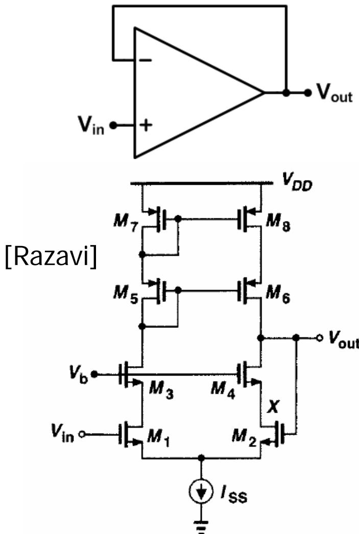
Minimum  $V_{out}$  set by M4 saturation
