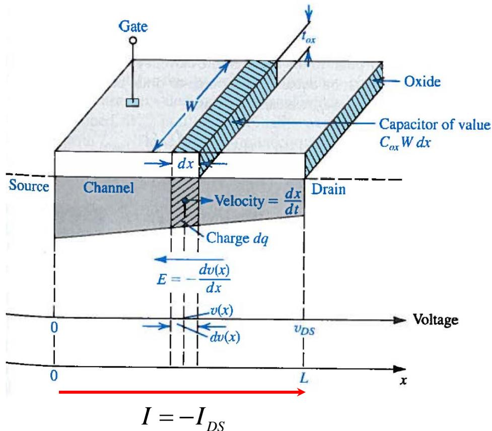
$$\text{Current from Source to Drain: } I = \frac{dQ}{dt} = \frac{dQ}{dx} \frac{dx}{dt} = Q_d(x)v$$
