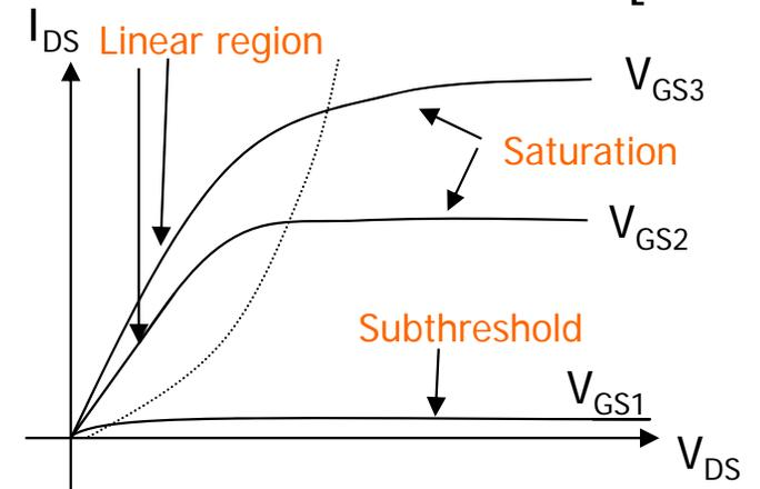
**Subthreshold** (extremely low-voltage low-power applications)
