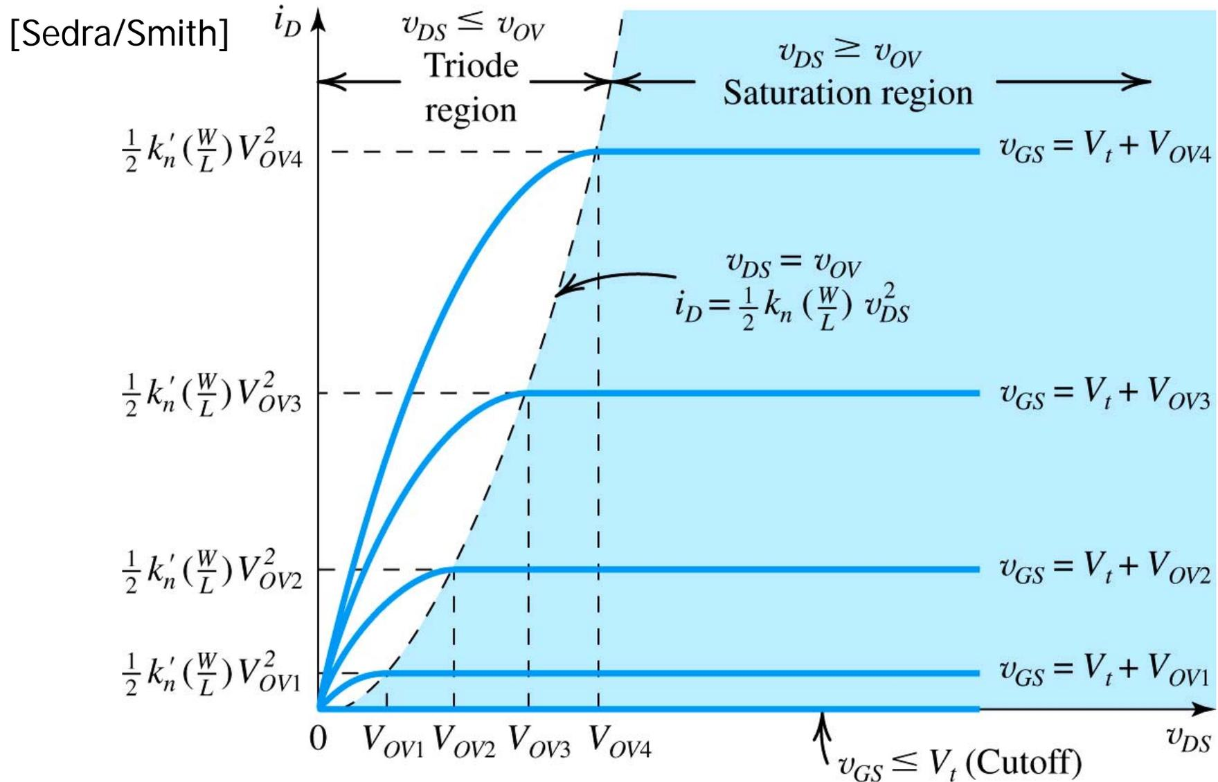
Note:  $V_{OV} = V_{GS} - V_T$  and  $k'_n = \mu_n C_{ox}$
