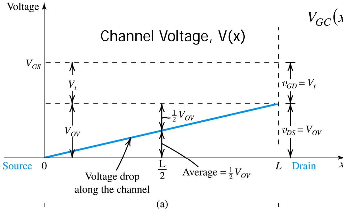
$$V_{GC}(x) - V_T = V_{GS} - V(x) - V_T = V_{OV} - V_{DS} \frac{x}{L}$$
