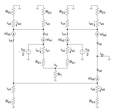
Figure 2: Small-signal circuit of the OTA.
