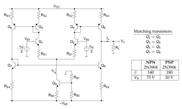
Figure 1: Operational transconductance amplifier (OTA) schematic.
