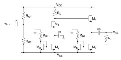
DC drain currents of  $M_1$  and  $M_4$  are set by the two current mirrors as follows:
