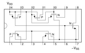
Note that all P-channel substrates are connected to  $V_{DD}$  and all N-channel substrates are connected to  $-V_{SS}$ .
