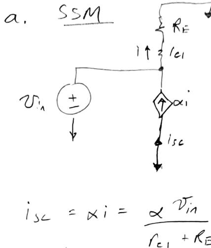
$$G_m = \frac{i_{sc}}{v_{in}} = \frac{\alpha}{r_{e1} + R_E} = \frac{g_{m1}}{1 + \frac{g_{m1} R_E}{\alpha}}$$
