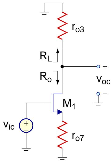
$$R_o = r_{o7} + r_{o1} + g_{m1}r_{o7}r_{o1}$$
