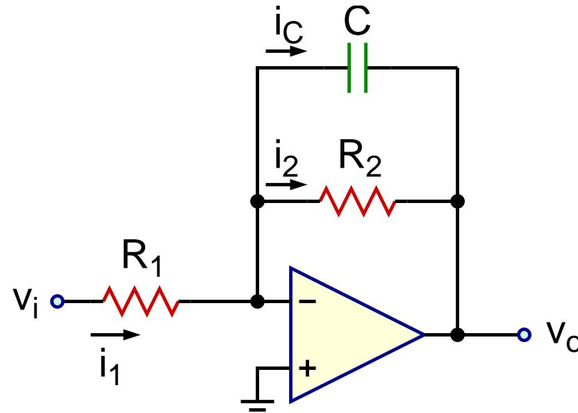
$$\frac{v_o}{v_i} = -\frac{\frac{R_2}{R_1}}{sR_2C + 1} = \frac{\kappa}{\frac{s}{\omega_o} + 1}, \quad \omega_o = \frac{1}{R_2C}, \quad \kappa = -\frac{R_2}{R_1}$$
