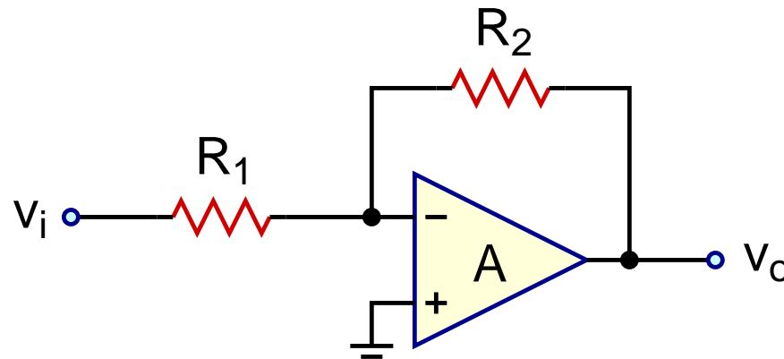
$$\frac{v_o}{v_i} = \frac{-\frac{R_2}{R_1}}{1 + \frac{R_2}{R_1}} A(s)$$
