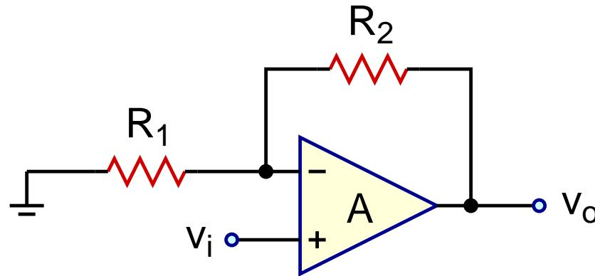
$$\frac{v_o}{v_i} = \frac{1 + \frac{R_2}{R_1}}{1 + \frac{R_2}{R_1} A(s)}$$
