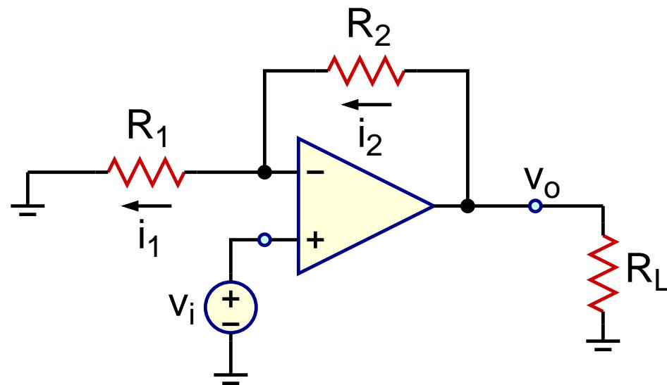
$$\frac{v_o}{v_i} = 1 + \frac{R_2}{R_1}$$
