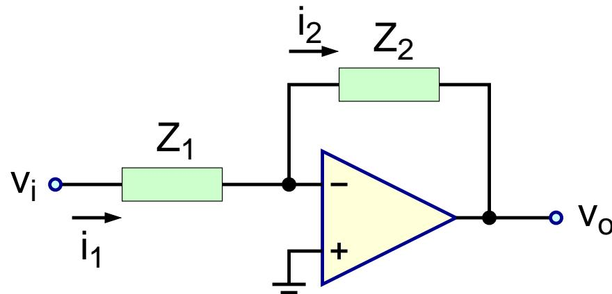
$$\frac{v_o}{v_i} = \frac{-\frac{Z_2}{Z_1}}{1 + \frac{(1 + \frac{Z_2}{Z_1})}{A}}$$
