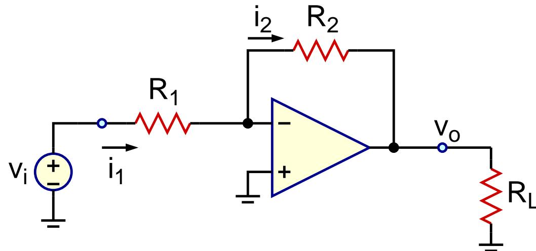
$$\frac{v_o}{v_i} = -\frac{R_2}{R_1}$$
