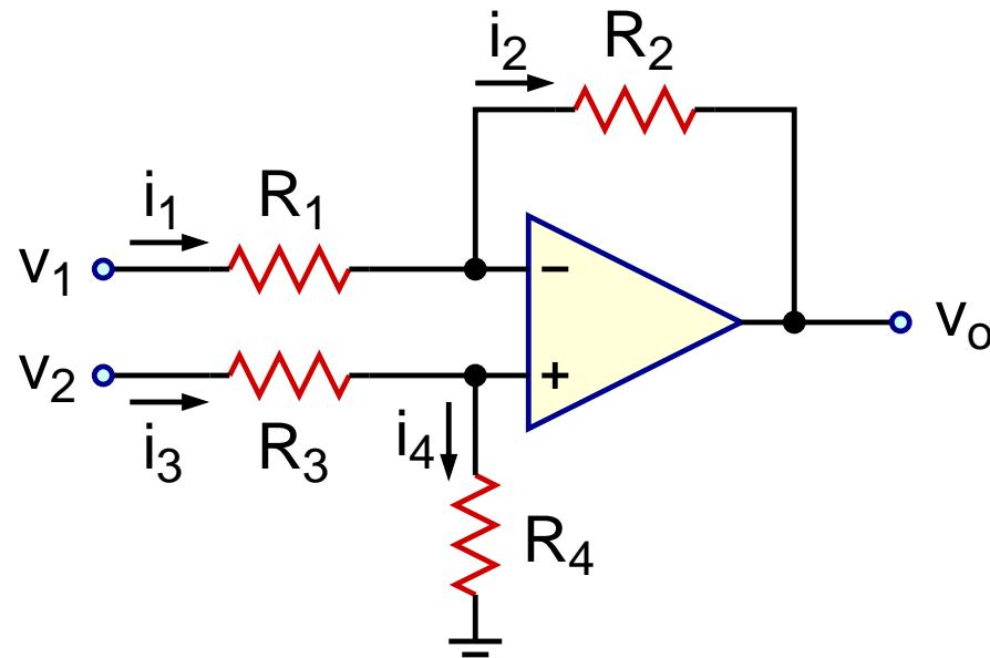
$$v_o = \frac{1 + \frac{R_2}{R_1}}{1 + \frac{R_3}{R_4}} v_2 - \frac{R_2}{R_1} v_1$$
