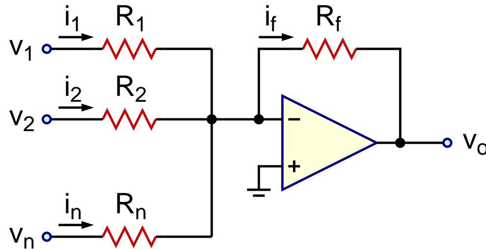
$$v_o = - \left( \frac{R_f}{R_1} v_1 + \frac{R_f}{R_2} v_2 + \cdots + \frac{R_f}{R_n} v_n \right)$$
