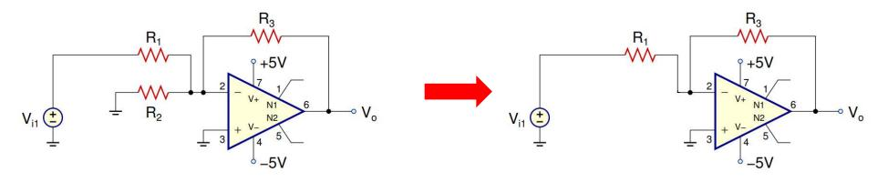
$$V_o = -\frac{R_3}{R_1} V_{i1}$$
