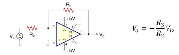
Now, due to the superposition theorem we can add the two inputs independently
