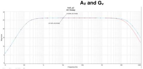
The simulated value of 26.2dB closely matches the hand calculation of 26.3dB for both  $A_v$  and  $G_v$ .
