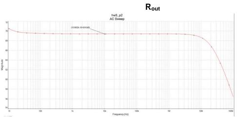
The simulated  $R_{out}$  value of 69.4dB $\Omega$  closely matches the hand calculation of 69.5dB $\Omega$ .
