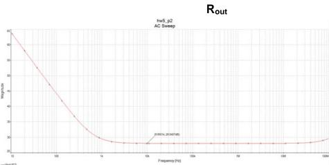
The simulated  $R_{out}$  value of 28.0dB $\Omega$  closely matches the hand calculation of 28.0dB $\Omega$ .
