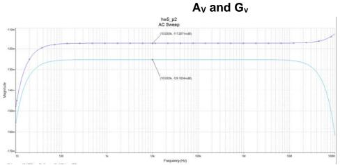
The simulated  $A_v$  value of -0.117dB matches closely the hand calculation of -0.114dB. The simulated  $G_v$  value of -0.125dB matches closely the hand calculation of -0.121dB.
