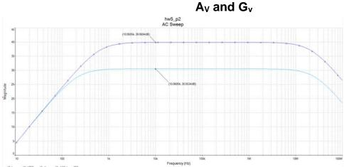
The simulated  $A_v$  value of 39.9dB matches closely the hand calculation of 40.3dB. The simulated  $G_v$  value of 30.6dB matches closely the hand calculation of 30.7dB.
