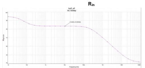
The simulated  $R_{in}$  value of 83.6dB $\Omega$  closely matches the hand calculation of 83.3dB $\Omega$ .
