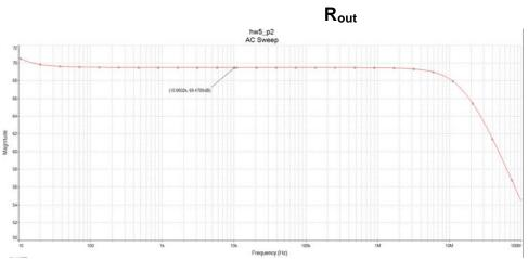
The simulated  $R_{out}$  value of 69.5dB $\Omega$  closely matches the hand calculation of 69.5dB $\Omega$ .
