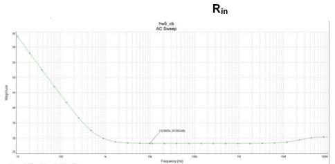
The simulated  $R_{in}$  value of 28.3dB $\Omega$  closely matches the hand calculation of 27.9dB $\Omega$ .
