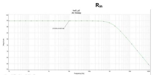
The simulated  $R_{in}$  value of 94.8dB $\Omega$  closely matches the hand calculation of 94.7dB $\Omega$ .
