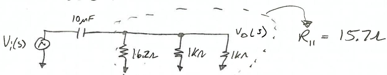
$$\frac{V_o(s)}{V_i(s)} = \frac{R_{II}}{\frac{1}{sC} + R_{II}} = \frac{s}{s + \frac{1}{K_{II}C}} = \frac{s}{s + 6.37 \times 10^3}$$
