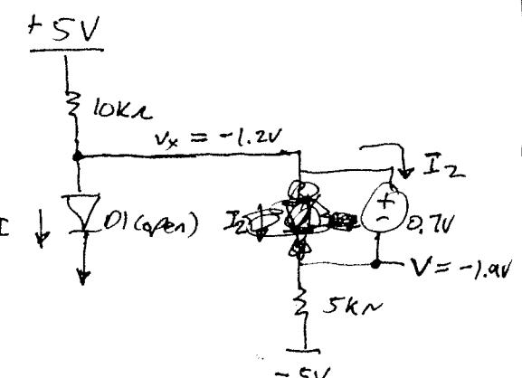
Case  $\phi 1 \Rightarrow D1 \text{ "ON" } \dot{\cup} \text{ } D2 \text{ "OFF" }$
