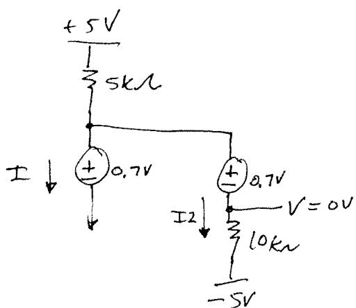
$$V_{D1} = V_{D2} = 0.7V$$
