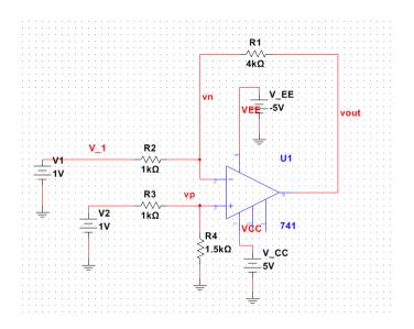
Set V2=1V and Sweep V1 from -0.5V to 0.5V. Notice that when V1=0, Vout=3V and the curve has a slope of -4V/V over the opamp's linear output range. Also notice that the opamp saturates at 4.1V, which is below the 5V positive power supply.
