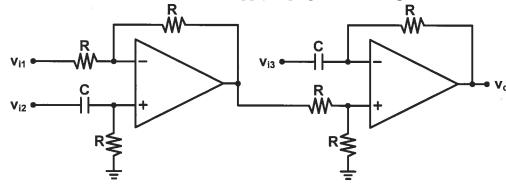
$$V_{0} = (-1)(\frac{1}{2})(1 + \frac{2R}{2c})V_{i1} + (\frac{2R}{2c+2R})(2)(\frac{1}{2})(1 + \frac{2R}{2c})V_{i2} - \frac{2R}{2c}V_{i3}$$
