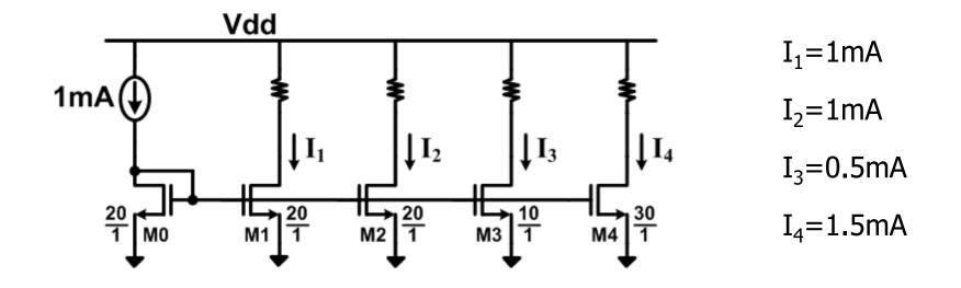
This bias scheme reduces sensitivity to process, voltage, and temperature variations
