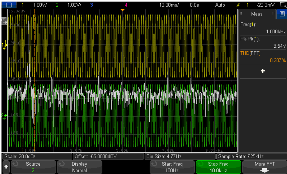
Figure 25: Total harmonic distortion window
