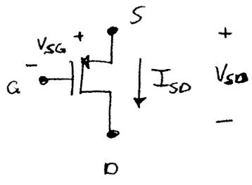
For Saturation:  $V_{SD} \geq V_{SG} - |V_{TP}|$
