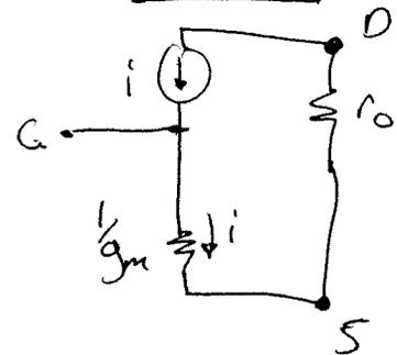
$$\text{NMOS: } g_m = \frac{\partial I_{D0}}{\partial v_{gs}} = K_{PN} \frac{W}{L} (v_{gs} - V_{TN}) = K_{PN} \frac{W}{L} V_{OD}$$
