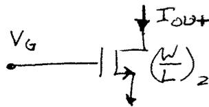
$$I_{out} = \frac{K_{PN}}{2} \left(\frac{W}{L}\right)_2 \left( \sqrt{\frac{2I_{REF}}{K_{PN} \left(\frac{W}{L}\right)_1}} + V_{TN} - V_{TN} \right)^2$$
