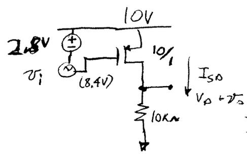
$$I_{SD} = \frac{1}{2} K_P \frac{W}{L} (V_{SG} - |V_{TP}|)^2$$
