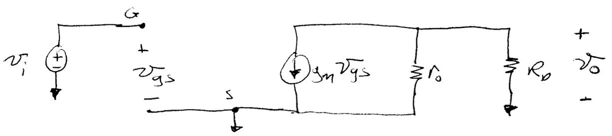
$$A_V = -g_m (R_D || r_o) = -540 \mu A/V (10 \text{ k}\Omega || 103 \text{ k}\Omega)$$
