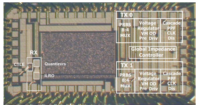
Fig. 19. I/O transceiver chip micrograph.
