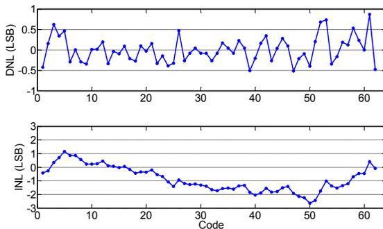
Fig. 10. DNL/INL plots with  $f_{in} = 2.7\text{MHz}$  at  $f_s = 1.6\text{GHz}$ .
