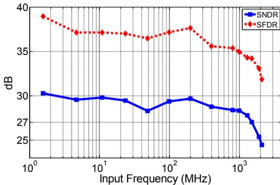
Fig. 9. ADC SNDR/SFDR vs. input frequency at  $f_s = 1.6\text{GHz}$ .
