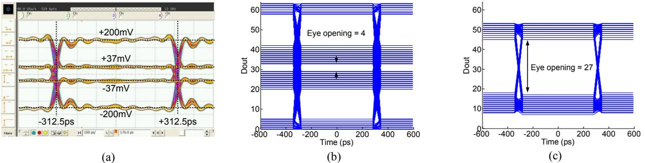
Fig. 8. (a) 1.6Gb/s ADC input generated by  $2^{23}-1$  PRBS after a 2-tap FIR with 15dB de-emphasis, and measured digitized 6b ADC output (b) without, and (c) with 1-tap DFE enabled.
