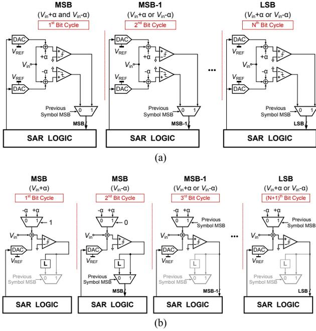
Fig. 3. Conceptual schematic of a unit SAR ADC with (a) loop-unrolled, and (b) proposed redundant cycle 1-tap embedded DFE.
