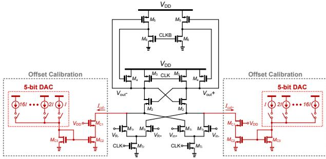
Fig. 6. Schematic of the 4-input comparator with offset calibration current DACs.
