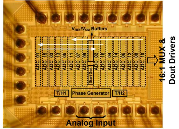
Fig. 7. Chip micrograph showing the position of unit ADCs and main building blocks.
