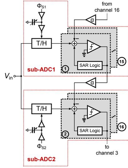
Fig. 4. Block diagram of the 16-way time-interleaved SAR ADC with embedded 1-tap DFE
