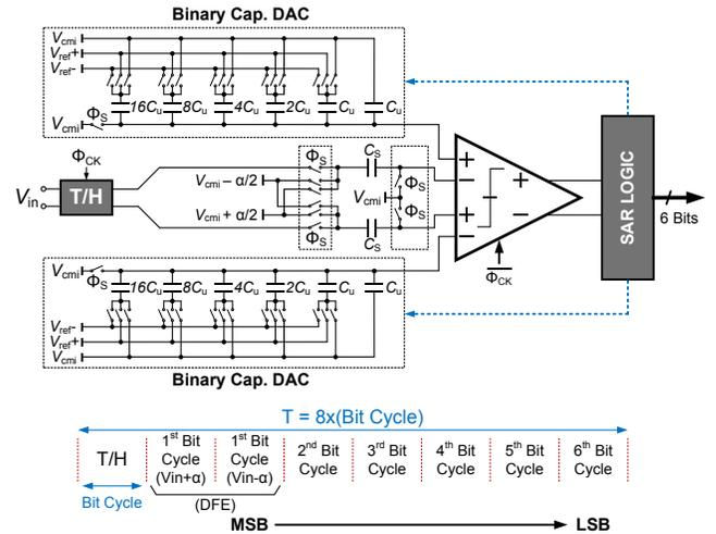
Fig. 5. Unit SAR ADC schematic with redundant cycle embedded 1-tap DFE.
