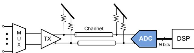
Fig. 1. A high-speed link with an ADC-based receiver.
