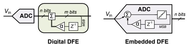
Fig. 2. Block diagrams of digital and embedded DFE.
