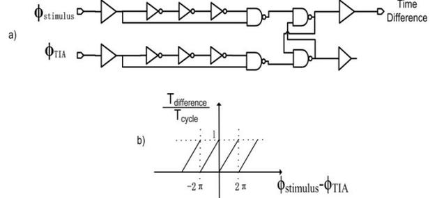
Figure 8. Phase detector: a) Schematic, b) Phase transfer characteristic.
