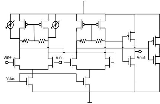
Figure 7. Comparator schematic.
