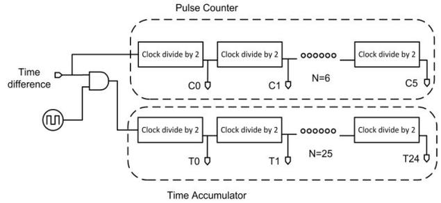
Figure 9. Divide-by-2 counter based TDC.
