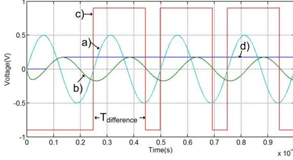
Figure 2. IS front-end operation: a) 40kHz stimulus signal ( $\times 50$ ), b) TIA output, c) Phase detector output, d) PDC output.
