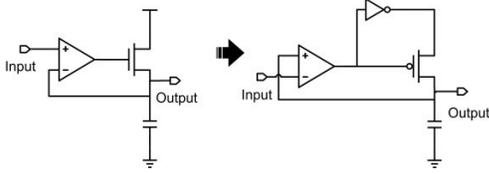
Figure 5. Peak detector circuits: a) Conventional NMOS topology b) Proposed PMOS version.
