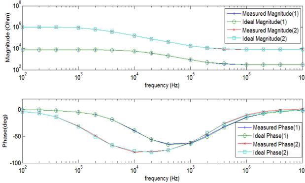
Figure 11. IS front-end cell model measurements.
