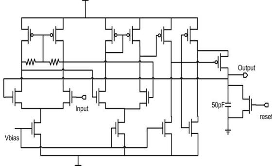
Figure 6. Detailed PDC schematic.
