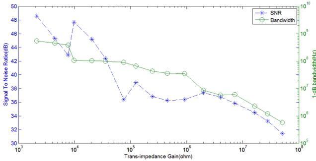
Figure 10. TIA bandwidth and output SNR.
