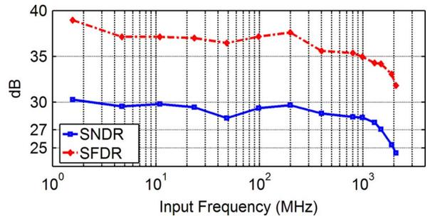
Fig. 14. ADC SNDR/SFDR versus input frequency at  $f_s = 1.6$  GHz.
