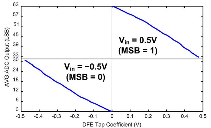
Fig. 17. Measured DFE tap coefficient range and resolution using a dc input voltage.
