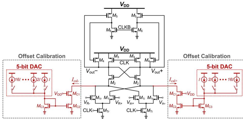
Fig. 10. Schematic of the four-input comparator with offset calibration current DACs.
