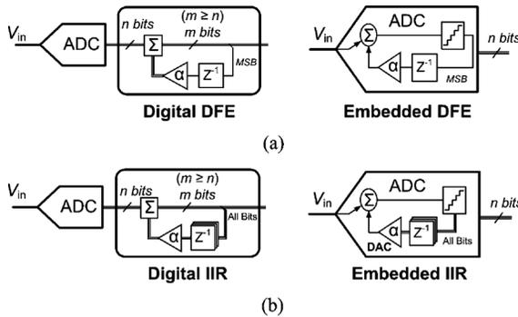
Fig. 2. Block diagrams of (a) digital versus embedded DFE and (b) digital versus embedded IIR.
