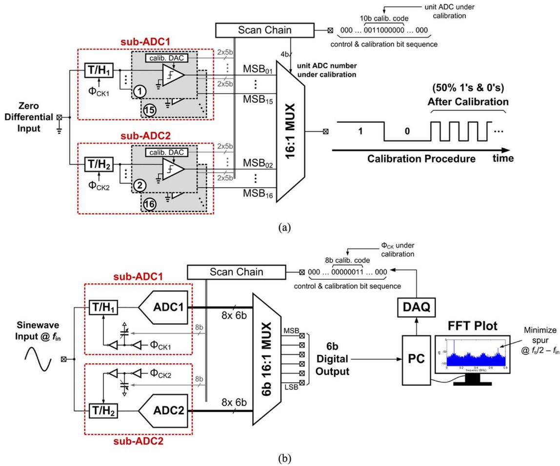
Fig. 12. Simplified diagrams of the foreground (a) offset calibration and (b) clock skew calibration setups.
