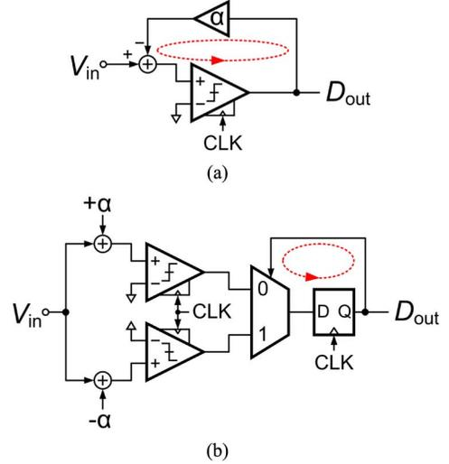
Fig. 4. DFE implementations. (a) Direct-feedback. (b) Loop-unrolled.
