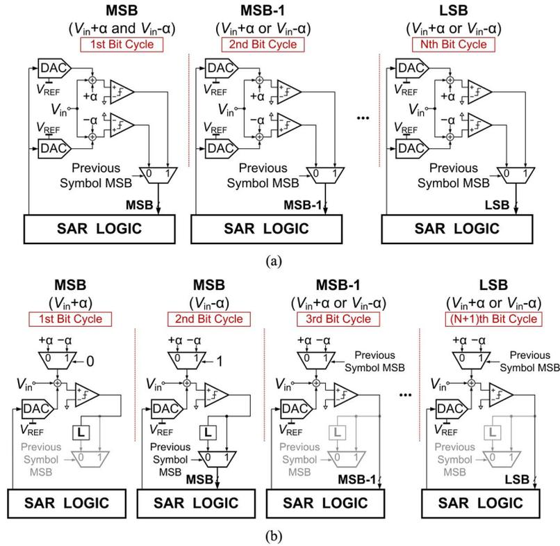
Fig. 5. Conceptual schematic of a unit SAR ADC with (a) loop-unrolled and (b) proposed redundant cycle one-tap embedded DFE.
