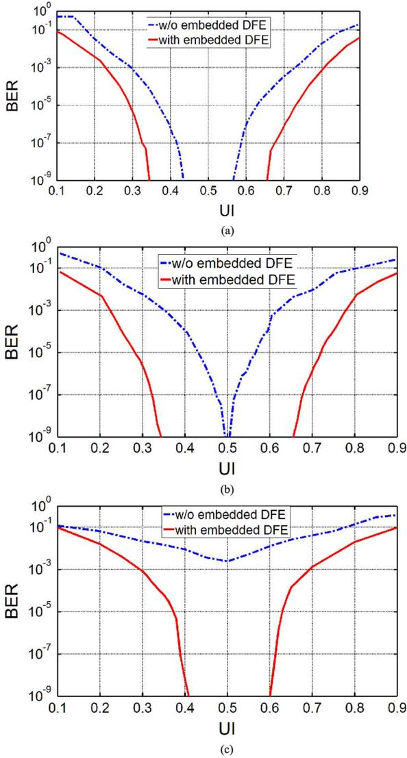
Fig. 19. Measured bathtub curves for the (a) 30-in smooth, (b) 28-in notch, and (c) 46-in higher loss FR4 channels shown in Fig. 3, with and without one-tap embedded DFE for a  $2^{10} - 1$  PRBS input with 1- $V_{pp}$  TX swing and no TX equalization.
