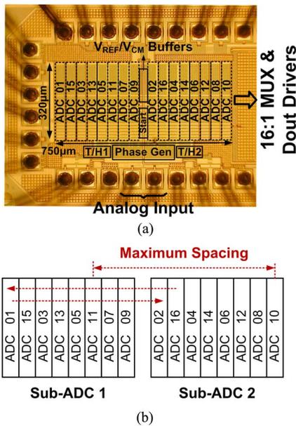
Fig. 13. Prototype ADC implemented in an LP 90-nm CMOS process. (a) Chip micrograph. (b) Optimized order of unit ADCs with respect to spacing between each two consecutive ADCs.
