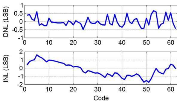
Fig. 16. DNL/INL plots with  $f_{in} = 2.7$  MHz at  $f_s = 1.6$  GHz.
