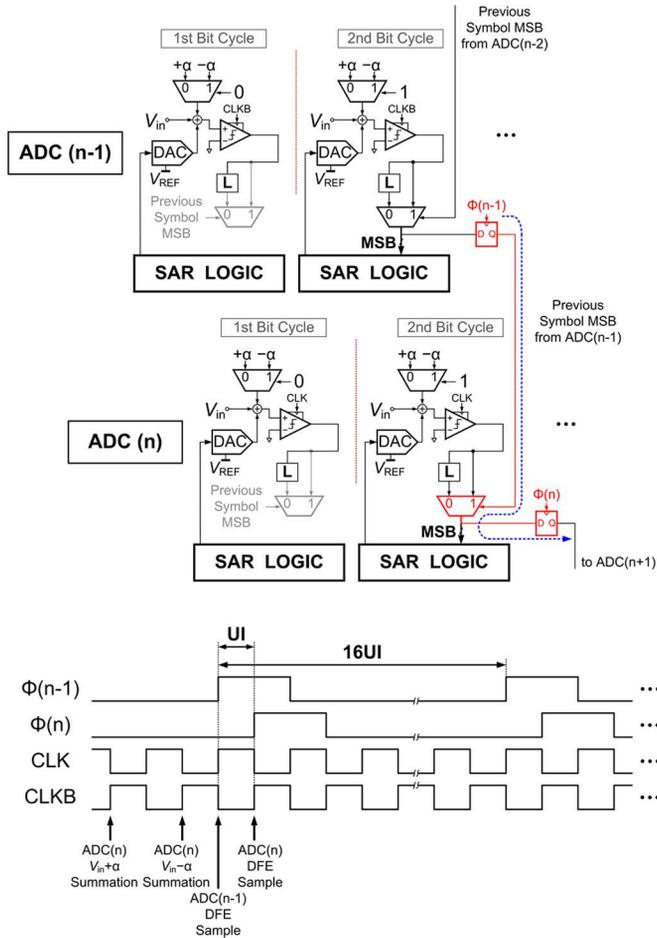
Fig. 6. Critical delay path for the redundant cycle one-tap embedded DFE. The instants when the summation and sampling in the one-tap embedded DFE occur are shown.
