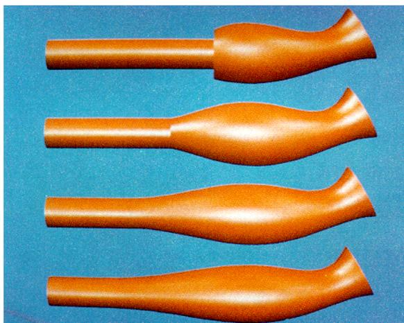
Fig. 12  $C^{-1}$ ,  $C^0$ ,  $C^1$  and  $C^2$  Local Deformations
