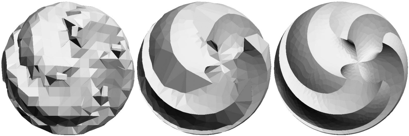
Figure 1: Left: initial 30^3 marching cubes mesh, 2.9K triangles. Middle: mesh optimized without adaptive subdivision (2.9K triangles), see Section 2 for details. Right: mesh optimization with adaptive subdivision was used (20K triangles), see Section 3 and Table 1 for details.
