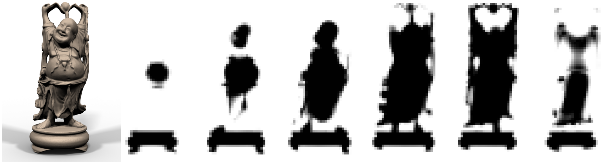
Figure 1: Slices from a 3D rasterization of the Happy Buddha statue computed on a 64^3 grid to illustrate the anti-aliased nature of wavelet rasterization.
