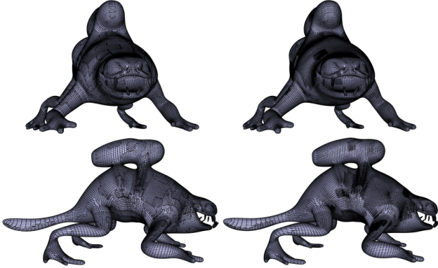
Figure 8. View dependent tessellation using rational sampling (top left) and exponential, subdivision sampling (top right). An alternate view of the same tessellation (bottom).
