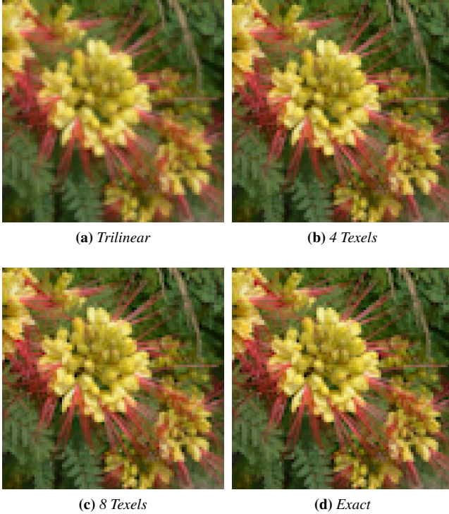
Figure 9: We show images downsampled using (a) trilinear interpolation, our approximation of the Lánczos 2 filter using (b) 4 and (c) 8 texels, then (d) exact evaluation of the Lánczos 2 filter.
