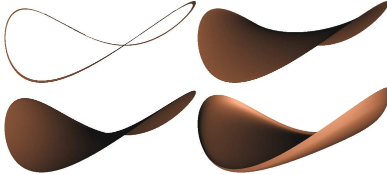
Fig. 2. Examples of interpolants created for an ellipse with a height function v_1^2 - v_2^2 specified on the boundary. The interpolants correspond to k = 0 on the top row and k = 1, 2 on the bottom row.
