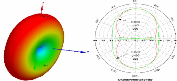
Figure 4. 3-D and 2-D far-field radiation plots.
