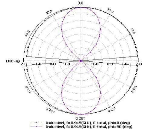
Fig. 5 Radiation pattern display of the antenna with arc-shape arms, directivity=1.99dBi
