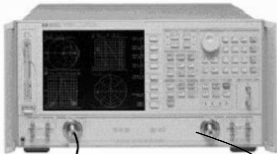
Network S-parameter analyzer (HP8719ES)
