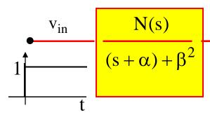
$v_{o_s}(t) = K_1 + K_2 e^{-\alpha t} \sin(\beta t + \theta)$
