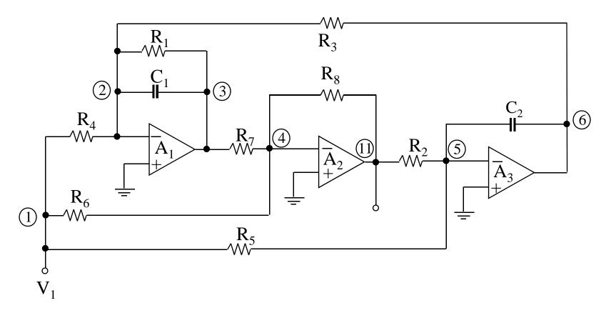
Analysis using KCL at the input of A1 plus the simple relations of V11/V3 and V6/V11 yields the following transfer function.
