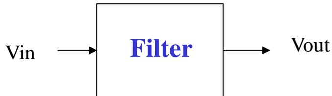
$$v_{\text{out}}(t) = K v_{\text{in}}(t - t_0)$$
