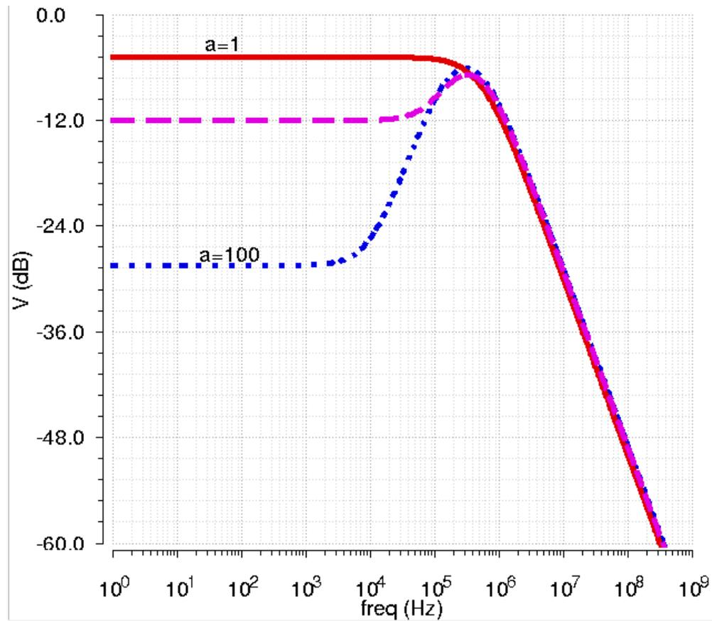
Figure 3: Filter Simulation for different values of a
