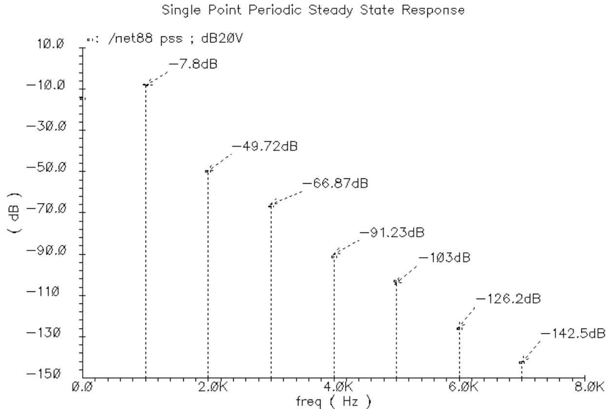
$$V_{out} = a_o + a_1 v_d + a_2 v_d^2 + a_3 v_d^3 + a_4 v_d^4 + a_5 v_d^5 + a_6 v_d^6 + a_7 v_d^7$$
