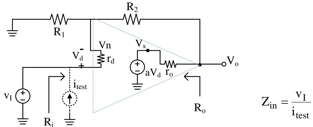
$$Z_{in} = \frac{v_I}{i_{test}}$$
