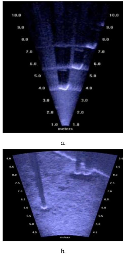
Fig. 4. DIDSON imagery: a.) shows no scour at Rollover Pass Bridge after Hurricane Ike, b.) shows scour (dark “holes” in front of pilings) at Marco Island dock after Hurricane Wilma.
