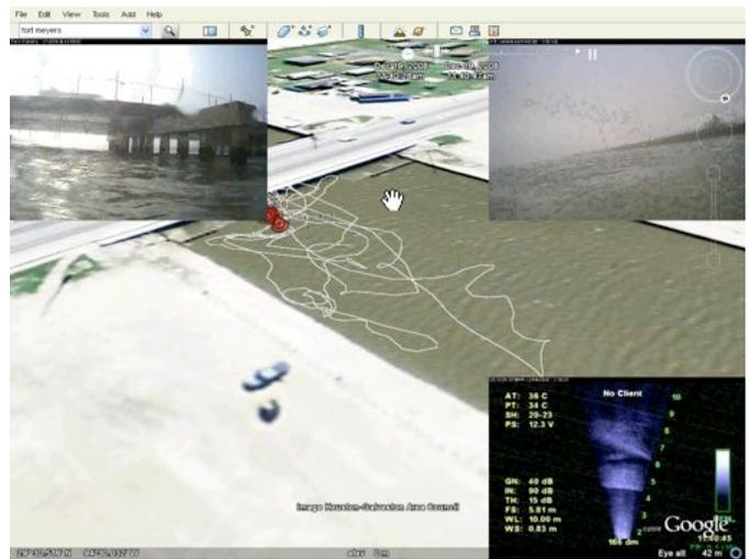
Fig. 2. Interface showing satellite imagery of the Rollover Pass Bridge with overlays of Sea-RAI camera and sonar views.
