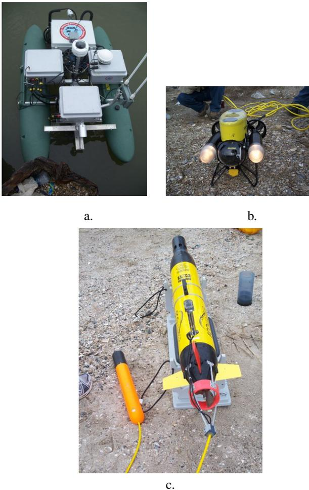
Fig. 3. Three UMVs used: a) Sea-RAI USV, b) VideoRay tethered ROV, and c) YSI Ecomapper autonomous UUV.
