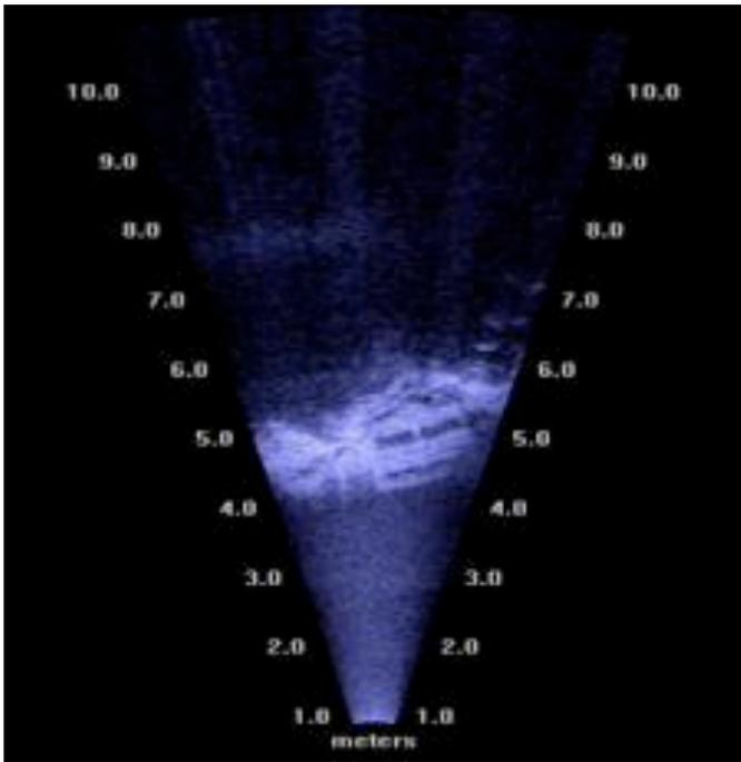
Fig. 5. DIDSON imagery: pallet in the debris in the channel.
