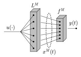
Figure 1: Architecture of an LSM. A function of time (time series)  $u(\cdot)$  is injected as input into the liquid filter  $L^M$ , creating at time t the *liquid state*  $x^M(t)$ , which is transformed by a memoryless readout map  $f^M$  to generate an output y(t).
