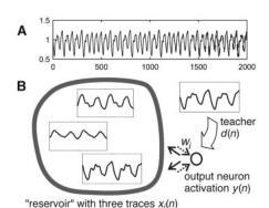
**Fig. 2.** (A) Prediction output of the trained ESN (dotted) overlaid with the correct continuation (solid). (B) Learning the MG attractor. Three sample activation traces of internal neurons are shown. They echo the teacher signal d(n). After training, the desired output is recreated from the echo signals through output connections (dotted arrows) whose weights  $w_i$  are the result of the training procedure.
