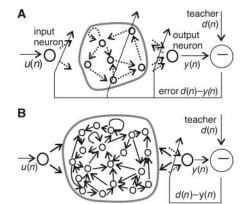
**Fig. 1.** (A) Schema of previous approaches to RNN learning. (B) Schema of ESN approach. Solid bold arrows, fixed synaptic connections; dotted arrows, adjustable connections. Both approaches aim at minimizing the error d(n) - y(n), where y(n) is the network output and d(n) is the teacher time series observed from the target system.
