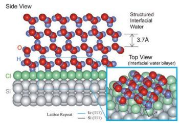
icon substrate. This ordered stacking persists for three to four bilayers ( $\sim 1$  nm) before disorientation takes place and results in crystallite islands, forming the layered structure. The size of atoms is not to scale for the van der Waals radii.
