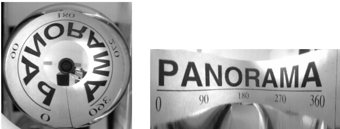
Figure 1. Omni-directional image captured by camera viewing convex mirror (left); same image reprojected onto cylindrical surface (right).
