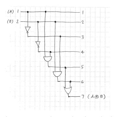
For the GA, generate some large initial population of random circuits using this circuit description language. To "cross" two circuits, cut them at the same random line of the circuit description and resplice the pieces to generate the two "offspring" to add to the population pool:
