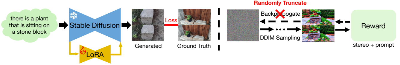
Figure 2. We show the overview of our approach comprising two stages (left and right). In the first stage, we fine-tune the pretrained Stable Diffusion model using LoRA [13] on our stereo image dataset, with left-right images stacked vertically. In the second stage, we further optimize our model using AlignProp [30] to enhance the stereo consistency and prompt alignment.
