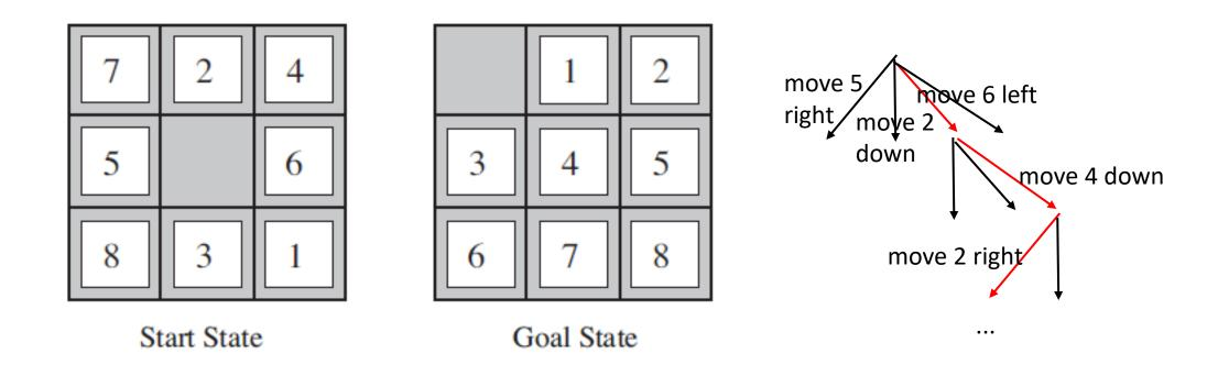
actions = slide a tile up/down/left/right into empty space a <u>solution path</u> is <u>sequence of actions</u> that transforms start state into the goal
